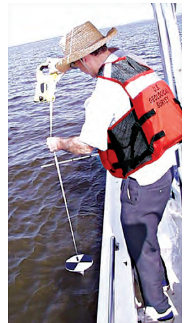
Figure 4-8. Measuring water clarity using a Secchi disk. Photo by U.S. Geological Survey.
