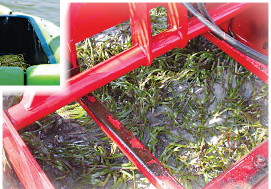
Figure 4–23. Seagrass sod (1.8 square meters) being excavated by Seagrass Recovery GigaUnit Transplant System, prior to transplanting. Photo by Penny Hall, Fish and Wildlife Research Institute.
