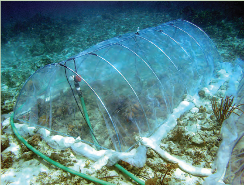
Box 4–1, Figure 1. The Submersible Habitat for Analyzing Reef Quality (SHARQ) benthic incubation chamber. This chamber consists of an aluminum frame covered by clear, flexible plastic-sheeting to trap water over the seafloor enabling scientists to analyze water chemistry using flow-through analytical systems. Photo by U.S. Geological Survey.
