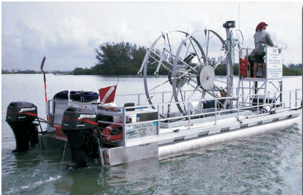
Figure 4–21. Mechanical seagrass planting boat developed and operated by Seagrass Recovery, Inc. This boat is called a “GigaUnit Transplant System” and was designed for the removal, transport, and replanting of large (1.8 square meters) planting units (or sods) of submersed aquatic vegetation along with the roots, rhizomes and associated sediments. Photo by Jim Anderson, Seagrass Recovery, Inc.
