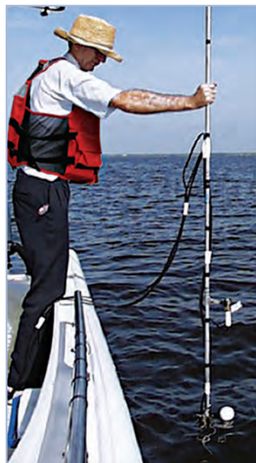
Figure 4-7. Measuring photosynthetically active radiation using quantum sensors. Photo by U.S. Geological Survey.
