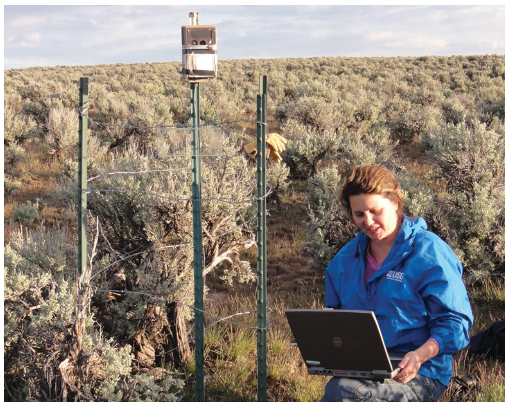
USGS scientist downloads data from phenocam located in Idaho. The phenocam takes a picture daily and that data is used to help track phenological changes (the timing and vigor of seasonal biological events). The data from the phenocam is used (with other data) to gain a better understanding of vegetation changes over the entire ecoregion. Photograph by USGS.
