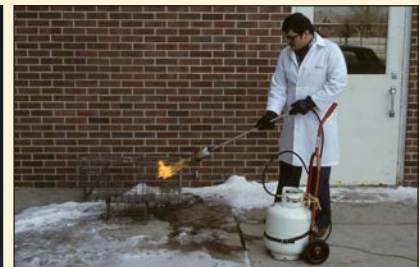
A. Propane flame gun (VT 3-30 Red Dragon Vapor Torch) with 20-pound gas tank. (Photo by Kevin Kazacos and Sam Royer)
