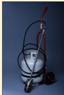
A. Propane flame gun (VT 3-30 Red Dragon Vapor Torch) with 20-pound gas tank. (Photo by Kevin Kazacos and Sam Royer)
