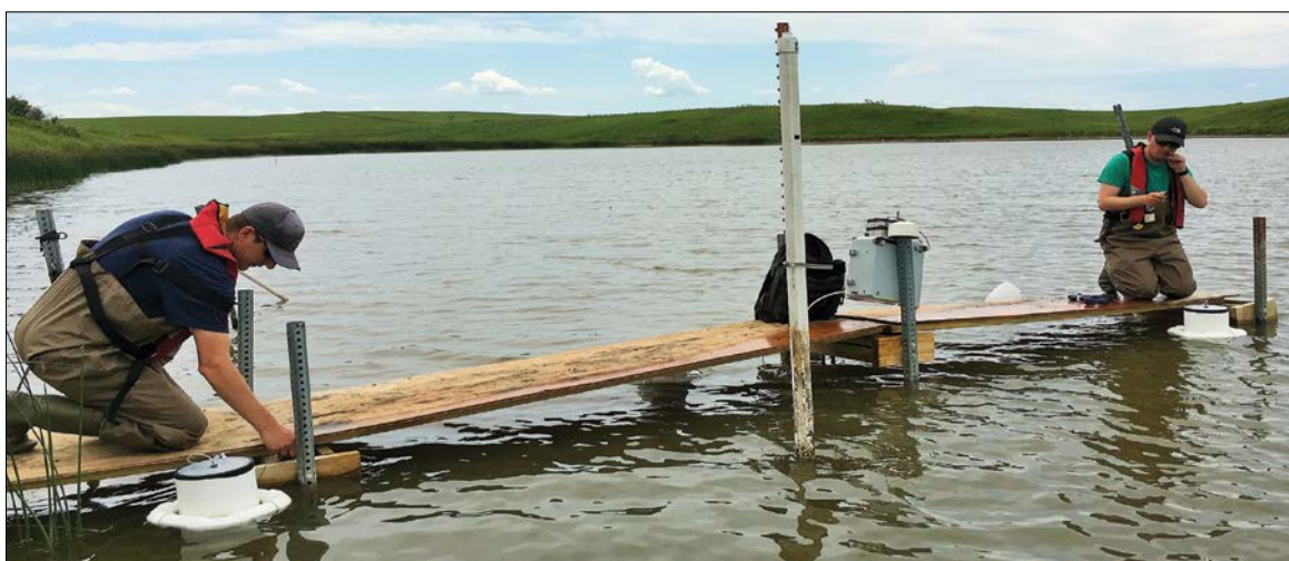
Technicians measuring greenhouse gas flux from floating chambers and water chemistry in a prairie pothole wetland at Cottonwood Lake Study Area, North Dakota (U.S. Geological Survey photograph).
