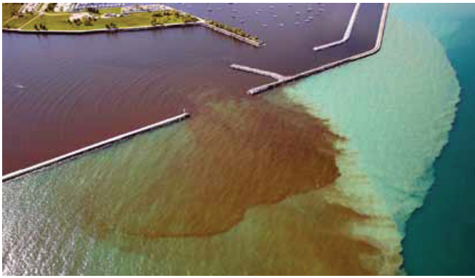
Figure 13. Combined sewer overflow event. (Source: Lyandres and Welch, 2012.)
