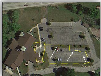
Willoughby Hills parking lot showing flow direction from impervious surface to permeable pavement perimeter. Source: Winston and others, 2015.
