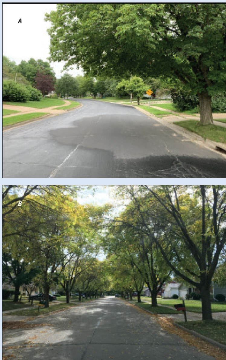
Figure S5.2. Photos showing, A , the effects of rainfall interception indicated by dry area underneath the canopy and, B , a tree lined street in Fond du Lac, Wisconsin. Trees intercept and store runoff and transfer water back to the atmosphere through evapotranspiration, reducing the volume of runoff. (Courtesy of U.S. Geological Survey.)
