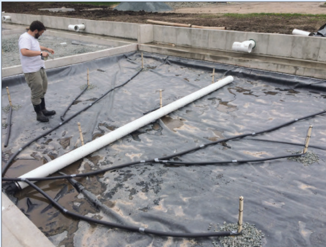
Figure S4.5. A network of temperature sensors placed in the porous asphalt test plot before installation of the aggregate base and asphalt surface. Attached to each wooden dowel placed in the three-by-three matrix were sensors spaced at about 0 (top), 6 (middle), and 12 (bottom) inches below the permeable surface. The pervious concrete and permeable interlocking pavers test plots had a similar configuration. (Source: Selbig and Buer, 2018.)
