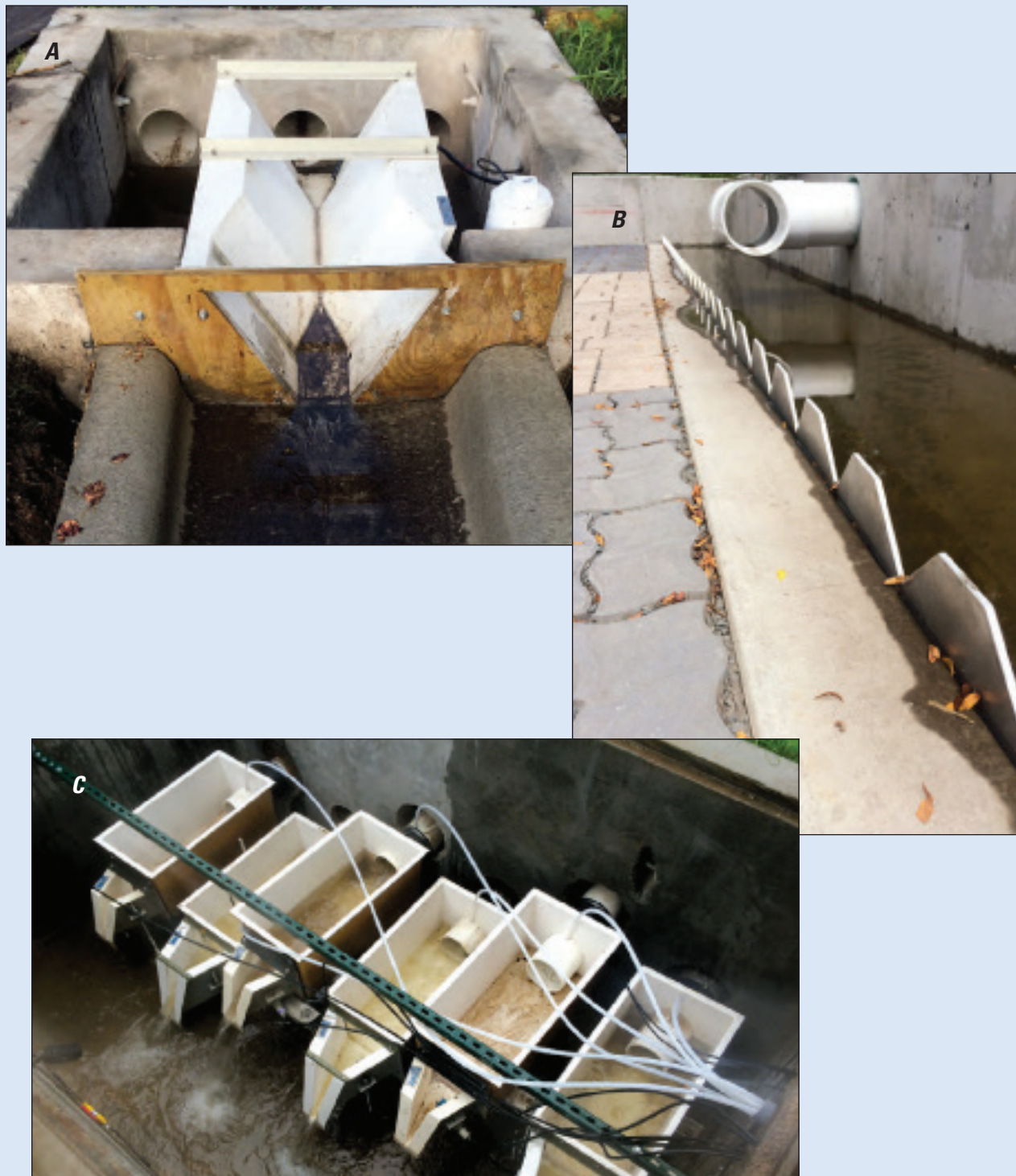
Figure S4.4. Hydraulic structures used to, A , measure and distribute the flow of runoff from the parking lot; B , uniformly spread runoff across the test surface; and, C , measure runoff that either passes through the underdrain of each permeable surface or bypasses as overflow. (Source: Selbig and Buer, 2018.)
