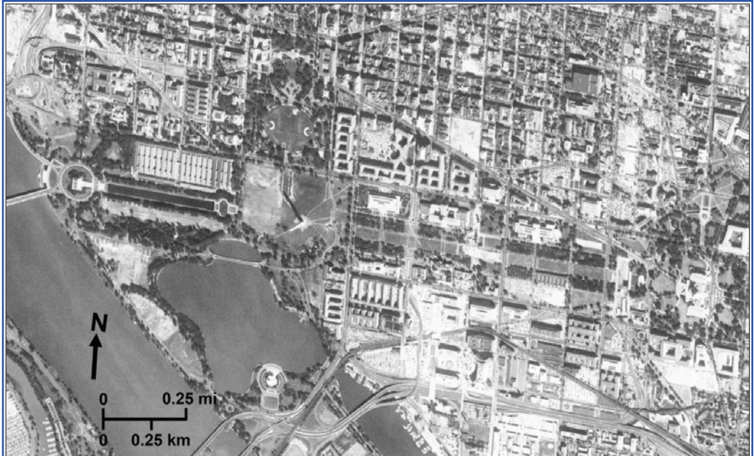
Figure 44. Corona satellite image of the National Mall, Washington, D.C.; Mission 1101, KH-4B camera. The image was acquired September 25, 1967, and the image resolution is 6 feet. The scale shown is approximate because the image is off-nadir (U.S. Geological Survey, 2017e).
