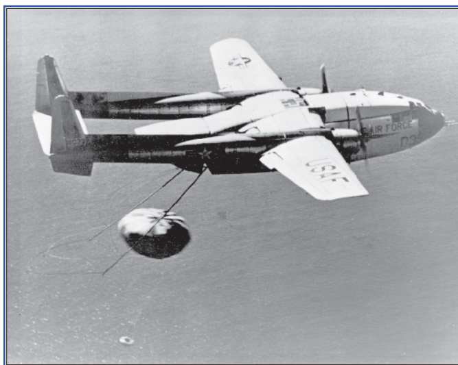
Figure 39. Photograph of a specially modified U.S. Air Force C-119J airplane recovering a Corona capsule returning from space. Photograph appears courtesy of the U.S. Air Force.
