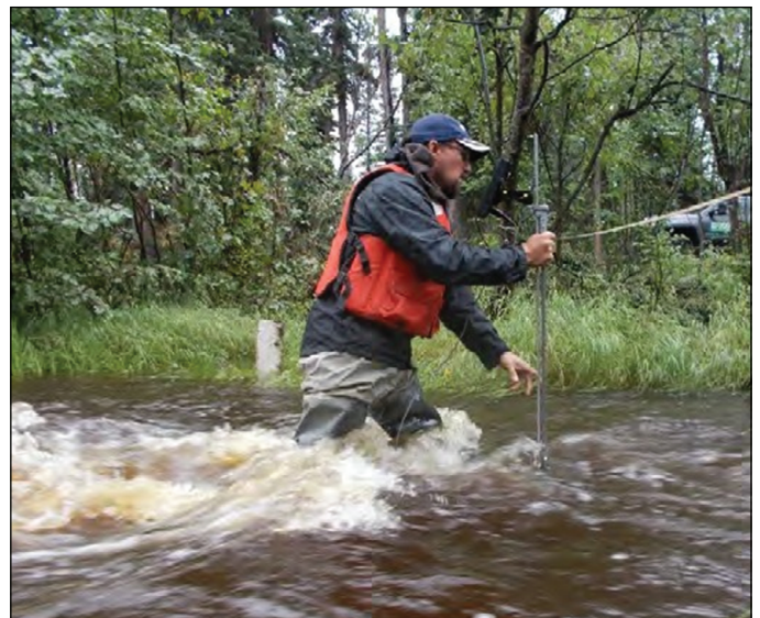
Photograph showing a U.S. Geological Survey technician measuring discharge during high flow at June Creek near Clear, Alaska. Photograph by Heather Best, U.S. Geological Survey.
