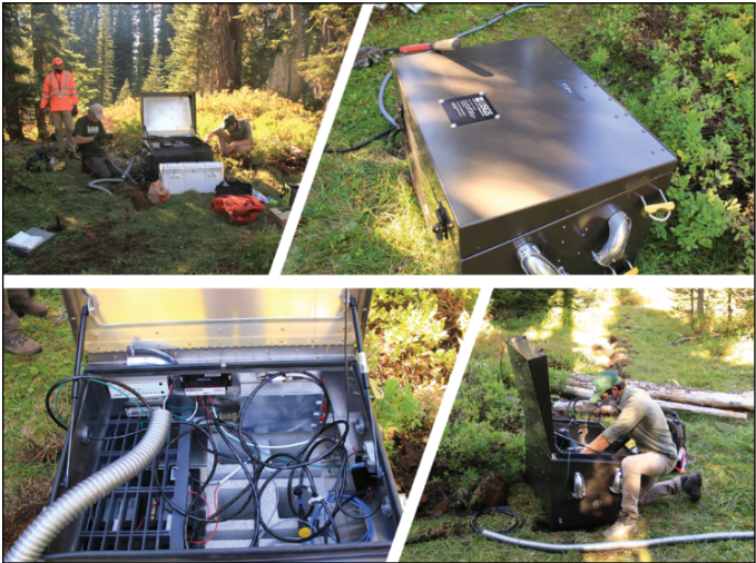
Photographs showing U.S. Geological Survey scientists installing a lahar detection system site at Mount Rainier, Washington. The secure box houses batteries, radio, and other equipment to detect lahars, power instruments, and return data to the U.S. Geological Survey Cascades Volcano Observatory. Detection algorithms automatically send alerts to emergency management centers in the Puget lowlands of Washington State. Photographs by Elizabeth Westby, U.S. Geological Survey.
