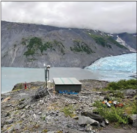
Photograph showing a ground-based synthetic aperture radar unit installed on the east side of Barry Arm, Prince William Sound, Alaska. This instrument is designed to capture high spatiotemporal resolution data by characterizing the motion of the Barry Arm landslide. Photograph by Dennis Staley, U.S. Geological Survey.
