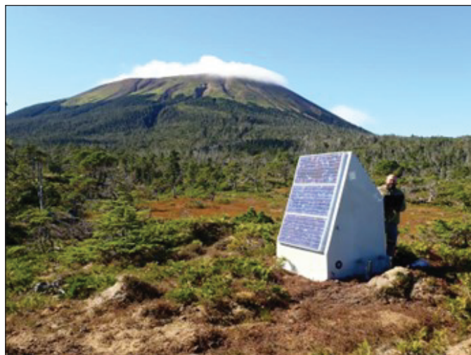
Photograph showing one of Alaska Volcano Observatory's three new seismic and Global Navigation Satellite System stations in a small network around the Mount Edgecumbe volcano in late fiscal year 2023. Shown is station EDES with Mount Edgecumbe in the background. Max Enders (U.S. Geological Survey) is pictured. Photograph by Max Kaufman, University of Alaska Fairbanks Geophysical Institute.
