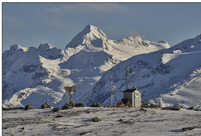
Photograph of the Wolverine Glacier weather station (U.S. Geological site number 15236895) on the Kenai Peninsula, with a weighing type precipitation gage with a large wind screen on the left, a radar-based precipitation sensor on the pole in the middle, and a new power system in the shack on the right. In the background are unnamed peaks on the edge of the Sargent Icefield.
