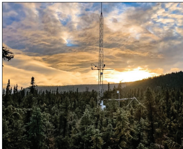
Photograph showing an eddy covariance tower at sunset continuously measuring the carbon balance of thawing permafrost ecosystems at the Alaska Peatland Experiment in the interior of Alaska. Photograph by Jack McFarland, U.S. Geological Survey.
