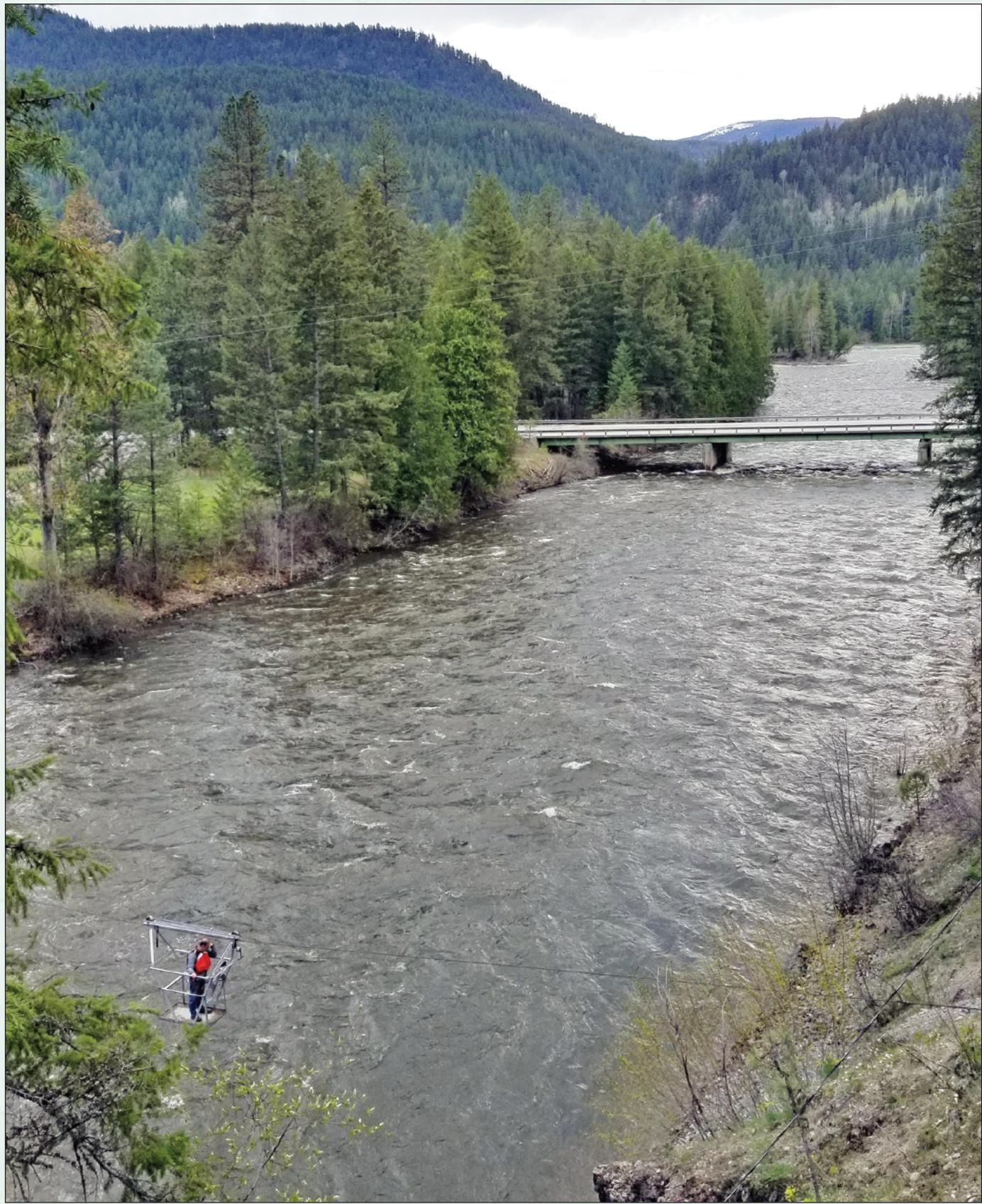
**Figure 23.** Photograph showing a U.S. Geological Survey hydrologic technician on the cableway over the Yaak River near Troy, Montana. Photograph by Ryan Smith, U.S. Geological Survey.
