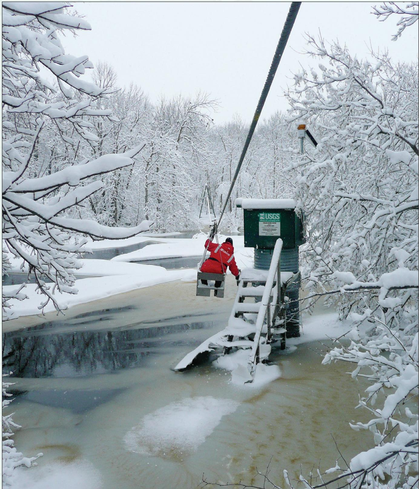
**Figure 18.** Photograph showing a U.S. Geological Survey (USGS) hydrologic technician using a cable car to access USGS streamgage 05104500 (Roseau River below South Fork near Malung, Minnesota) on March 26, 2009. Photograph by Brett Savage, USGS.
