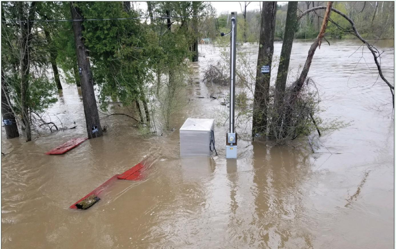
**Figure 15.** Photograph showing U.S. Geological Survey nutrient sampler submerged during major flooding on the Rifle River, Michigan, in May 2020. This site is near U.S. Geological Survey streamgage 04142000 (Rifle River near Sterling, Michigan). Photograph by Tom Weaver, U.S. Geological Survey.
