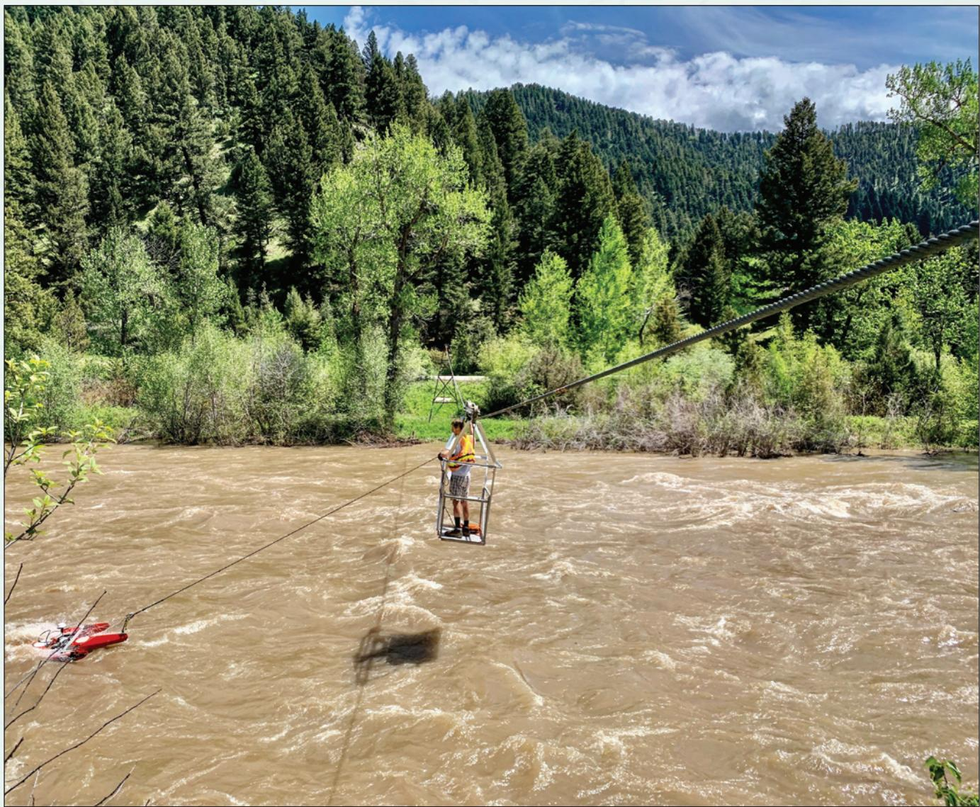
**Figure 6.** Photograph showing a hydrologic technician making a high-flow measurement during a snowmelt event on the Gallatin River near Gallatin Gateway, Montana. Photograph by Brett Price, U.S. Geological Survey.
