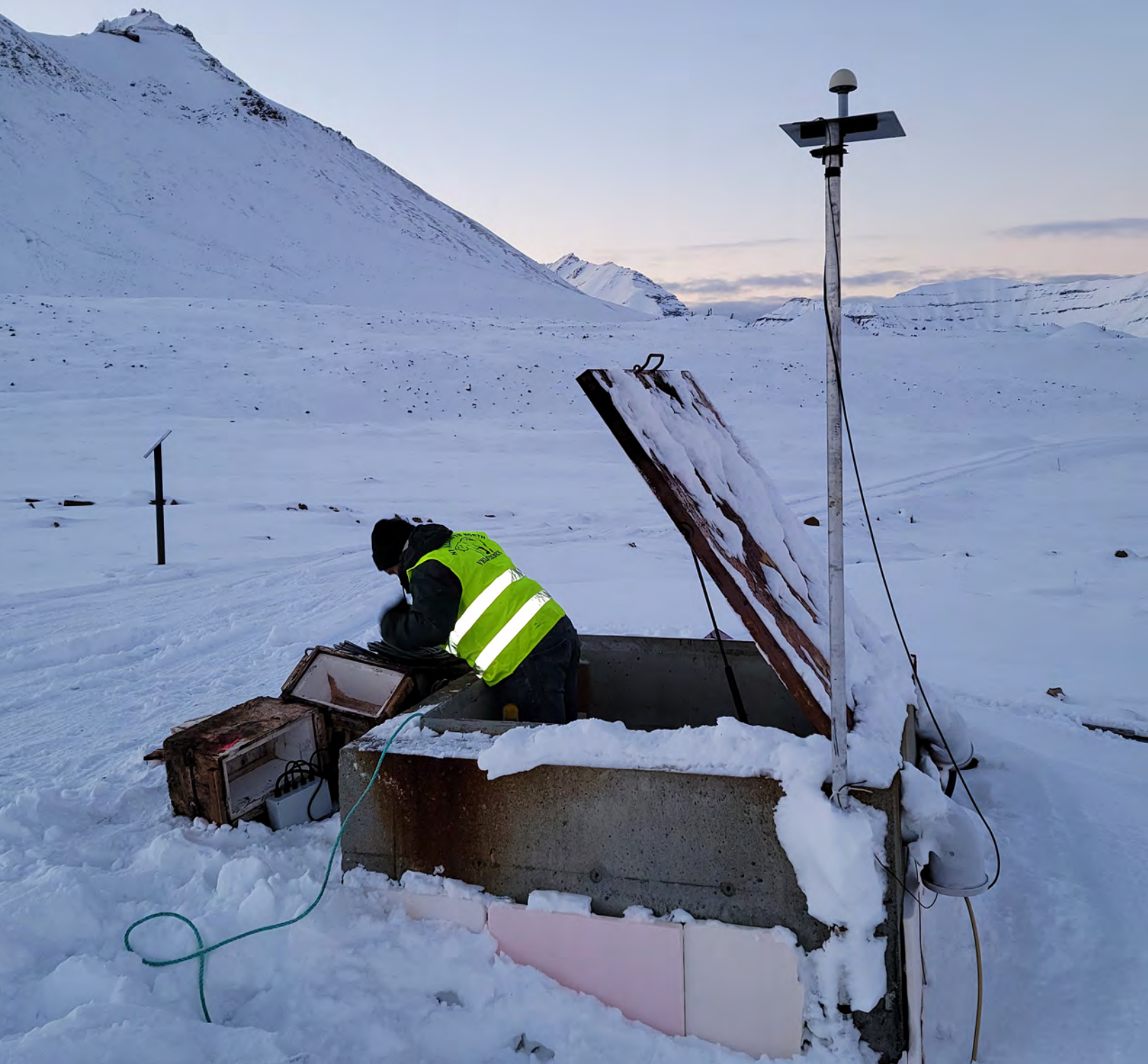
U.S. Geological Survey field engineer at the entrance of the underground vault at Global Seismographic Network station KBS in Ny-Alesund, Spitzbergen, Norway, October 26, 2022. Photograph by Jared Anderson, KBR.
