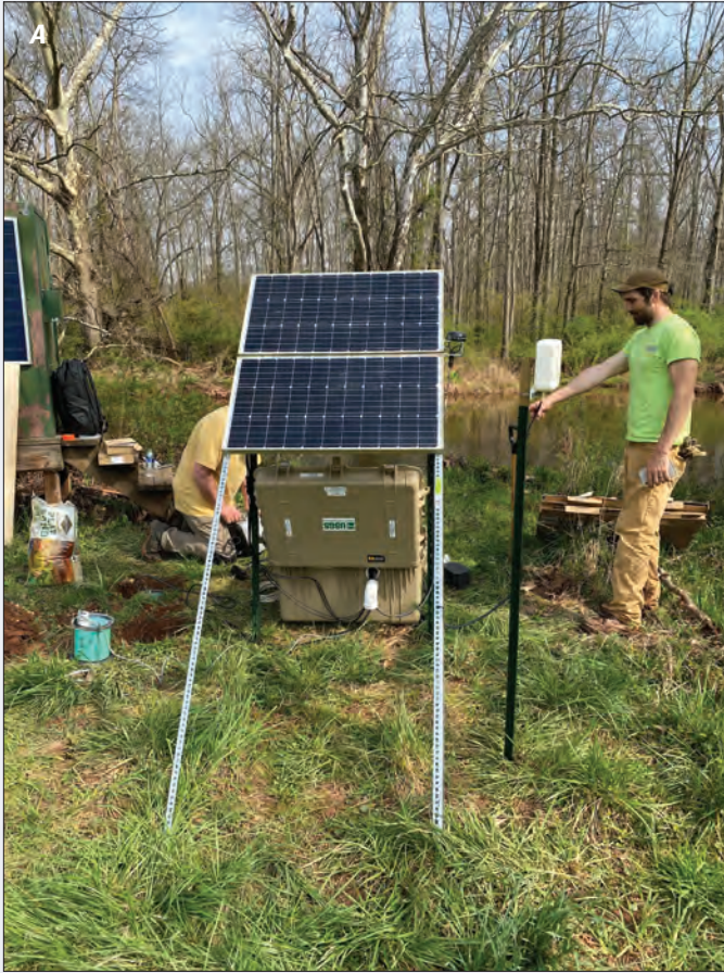
Figure 10. Example Albuquerque Seismological Laboratory (ASL) aftershock system. A , U.S. Geological Survey field engineers Greg Tanner (left) and Patrick Bowen (right) installing aftershock station NJ02 in response to the April 5, 2024, magnitude 4.8 earthquake in Tewksbury Township, New Jersey. Photograph by Steven Ploetz, U.S. Geological Survey. B , map of the five ASL aftershock stations (triangles) and aftershocks for the event (circles) with the number of stations used by the National Earthquake Information Center to locate the event indicated by color.
