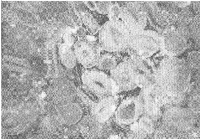
Figure 4.—Photomicrograph x 40 of polished surface of oolites in basal limestone of Sundance formation replaced by metatyuyamunite at locality 1. Light-colored oolites and parts of oolites, and white irregular deposits between oolites are metatyuyamunite.
