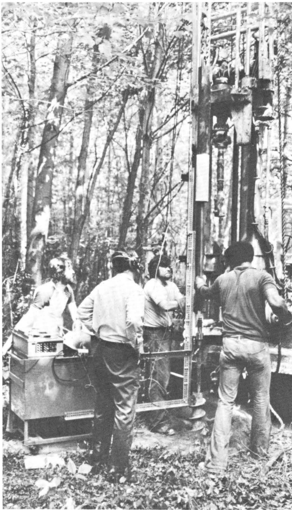
Field studies are being conducted to determine the energy delivered in the widely used standard penetration test.
