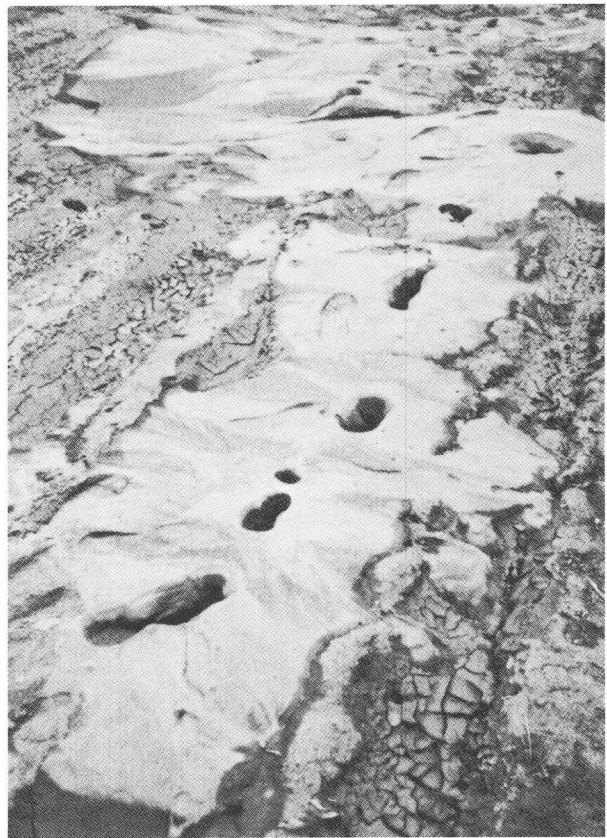
Typical liquefaction ground damage experienced in May 1983 earthquake near Tokoi, Japan.
