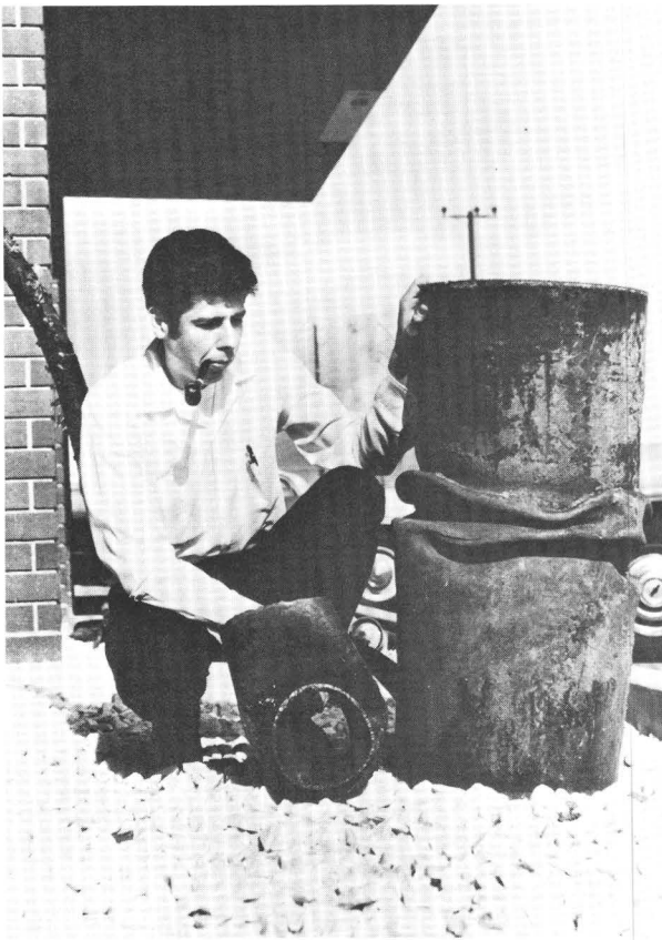
Pipeline, 16 inches in diameter, damaged during 1971 San Fernando earthquake.
