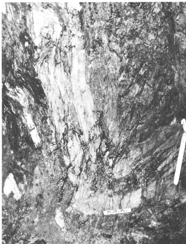
Figure 21.--Interbedded massive sulfide ore (dark layers of chalcopyrite and pyrite) and sandstone (light layers) in main stope of the Midas mine near Valdez. Study is part of U.S. Geological Survey investigation of ore deposits in Chugach National Forest. Photograph by S.W. Nelson.
