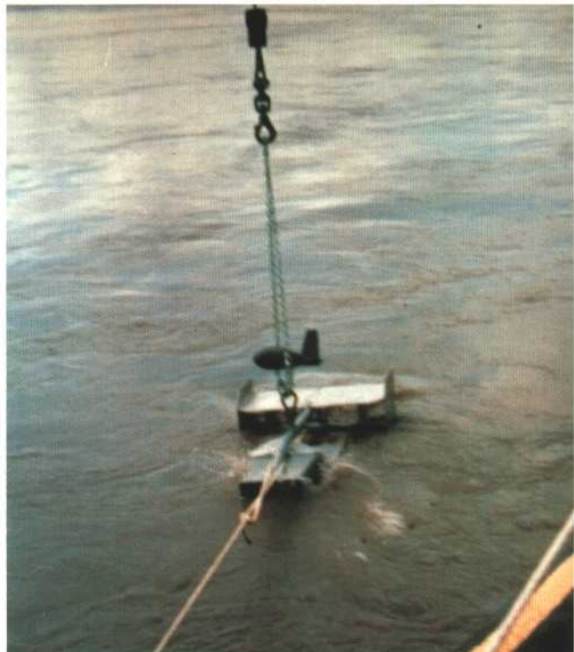
An attempt was made to collect bedload samples for the Mississippi River at St. Louis, Missouri, by using an experimental sampler designed at the U.S. Geological Survey Cascades Volcano Observatory, Vancouver, Washington. The sampler was suspended from a crane on the U.S. Army Corps of Engineers, St. Louis District, barge Pathfinder .
