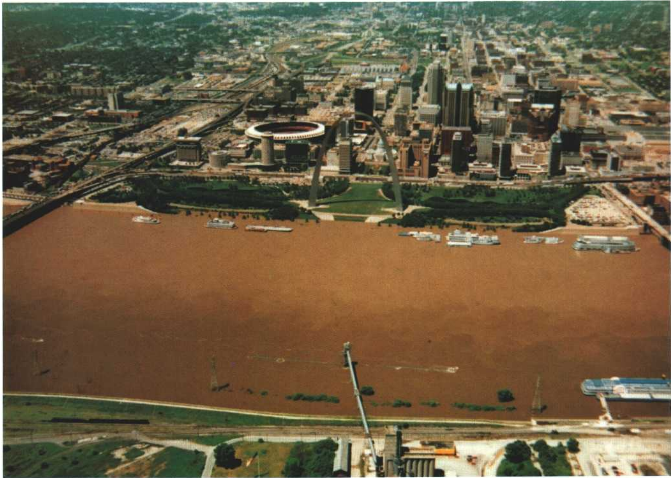
Figure 10. The Mississippi River at St. Louis, Missouri, July 30, 1993, looking west, showing the lateral variability in sediment concentration. Lighter areas are higher in suspended sediment, (Photograph from Srenco Photography, St. Louis, Missouri, 1993, and published with permission.)
