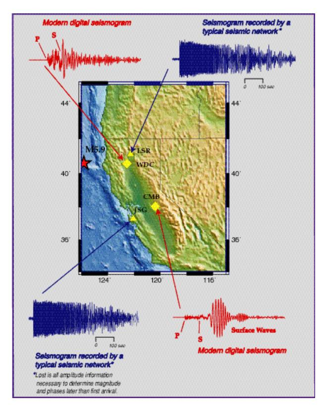
Obsolete seismic monitoring equipment dominates most seismic networks in the United States.
