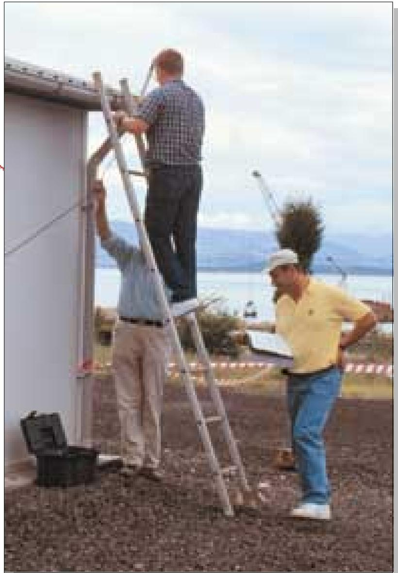
**Figure 29.** USGS scientists deploy an antenna for a portable seismic recording system at Dilovasi. Antenna receives time signals from a satellite and allows the timing on the portable seismographs to be synchronized with each other. *Photograph by Thomas L. Holzer.*
