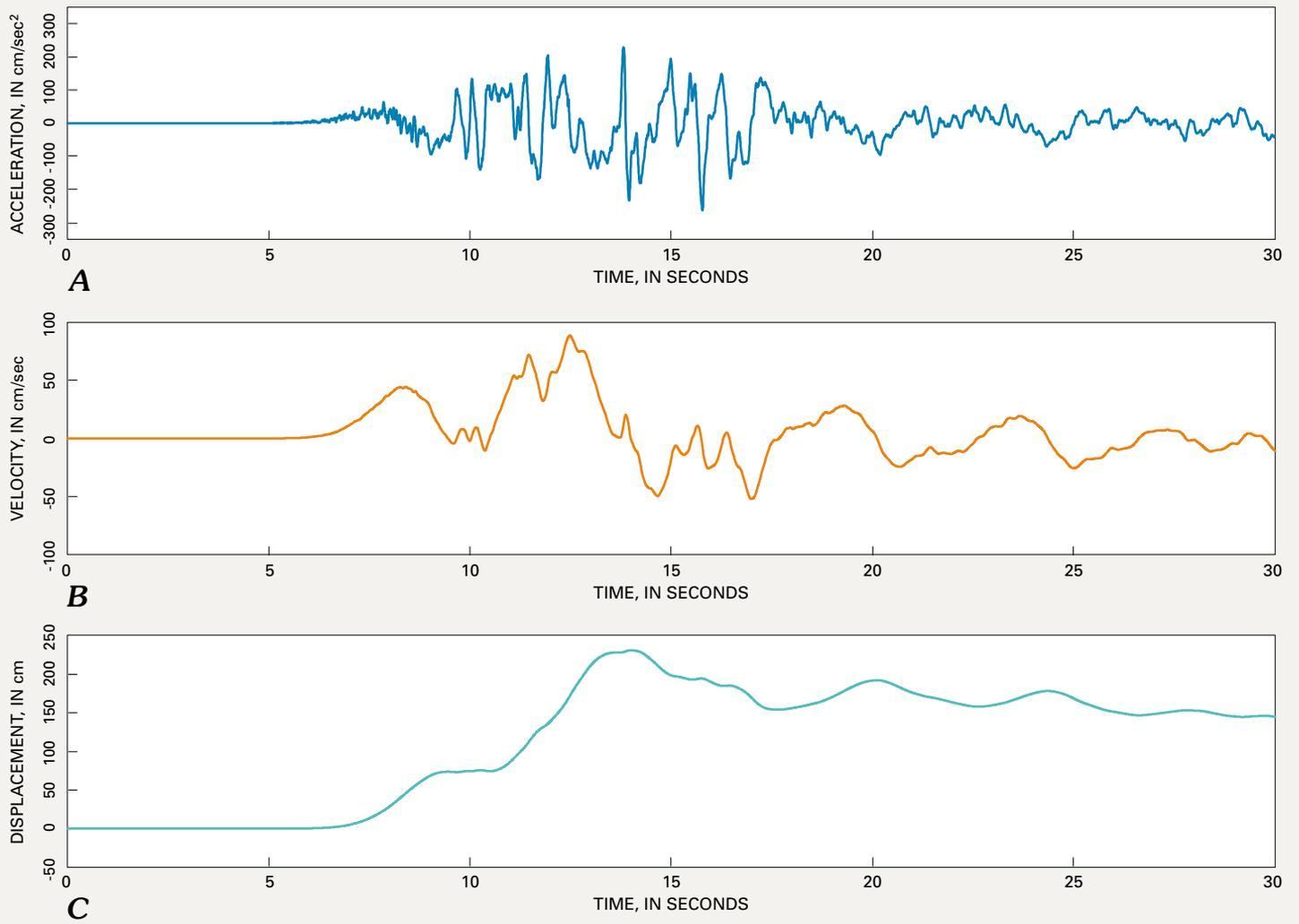
**Figure 4.** *A*, Recorded accelerations at the Kandilli Observatory and Earthquake Research Institute strong motion station, YPT, at the Petro-Chemical Plant in Korfez during the August 17, 1999, main shock. Station is about 4 km from the surface rupture. *B*, Velocities computed from acceleration time history showing large velocity pulse. *C*, Displacements computed for acceleration time history showing large displacement pulse. *Illustration by William L. Ellsworth.*
