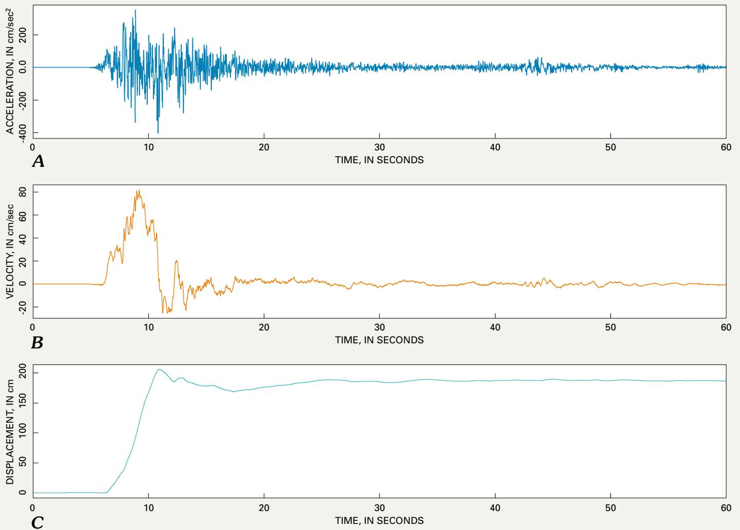
**Figure 3.** *A*, Recorded accelerations at the Turkish National Strong Motion Network station, SKR, in Adapazari during the August 17, 1999, main shock. Station is about 3.5 km from the surface rupture. *B*, Velocities computed from acceleration time history showing large velocity pulse. *C*, Displacements computed for acceleration time history showing large displacement pulse. *Illustration by William L. Ellsworth.*
