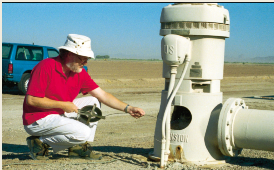
Measuring water level in dewatering well near Yuma, Arizona. Photograph by Sandra J. Owen-Joyce, U.S. Geological Survey.
