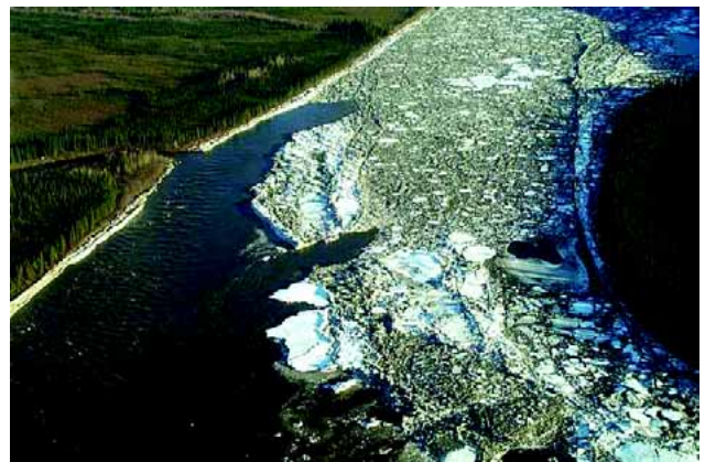
Ice jams, like this one on the Yukon River, Alaska, can cause severe flooding when impounded water overflows the stream channel upstream and when breakup of the jam suddenly releases water downstream. (Photograph courtesy of the Alaska Department of Military and Veterans Affairs)
