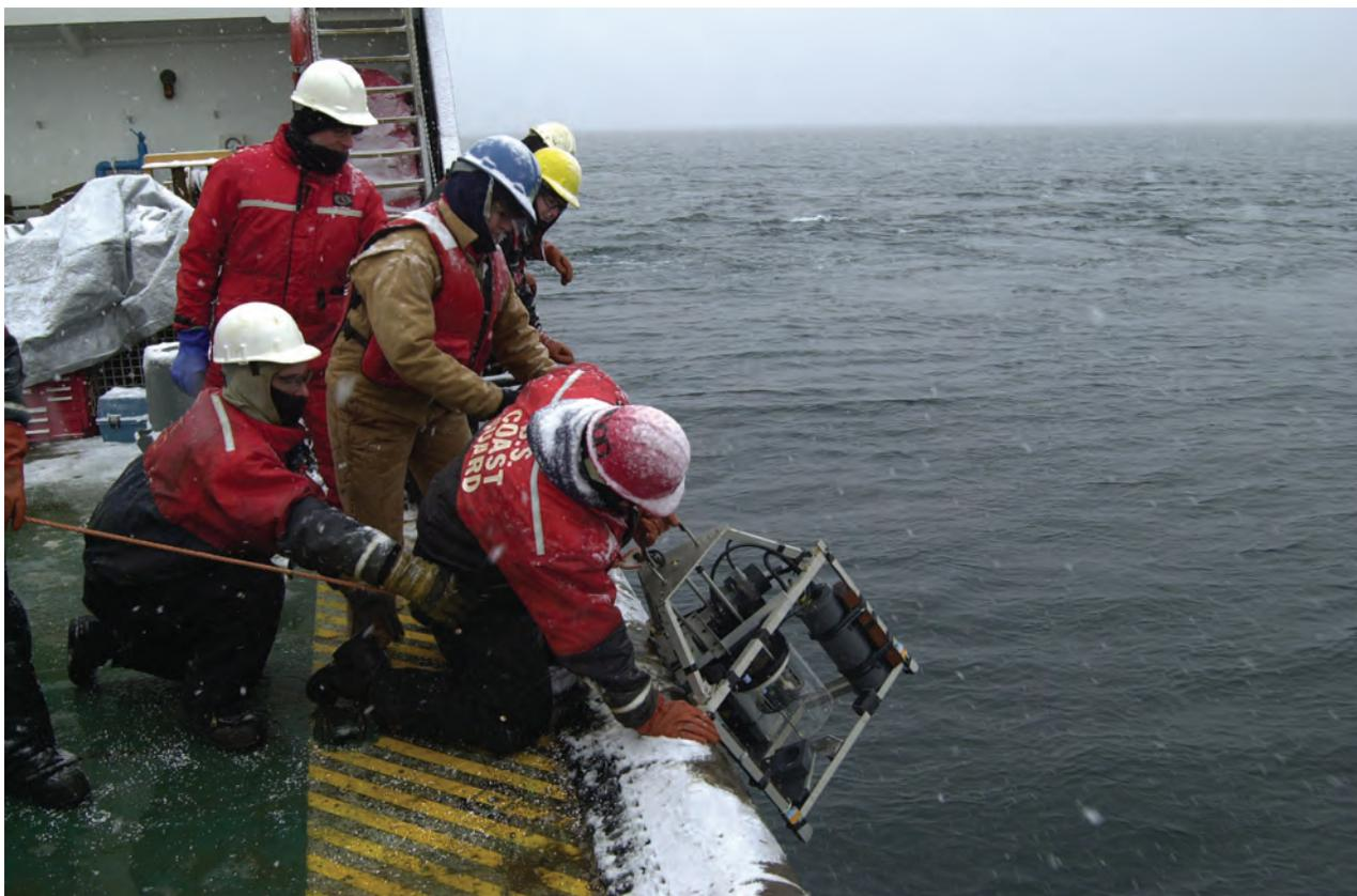
**Figure 8.1.** Winter recovery of the profiler on a typical February cruise. The clear plastic shroud in the center of the instrument houses the mobile sensor head on which are mounted the three electrodes and light sensor used to locate the sediment-water interface. Lending invaluable assistance are crew members of the U.S. Coast Guard Cutter *Marcus Hanna*.
