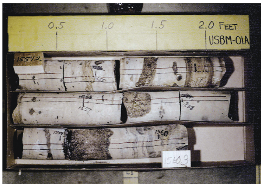
Figure 10. Drill core containing bands of light-brown nahcolite, small nodules of nahcolite, and nahcolite aggregates of bladed crystals in oil shale. Some nahcolite aggregates are rimmed with pyrite. Recovered core from the U.S. Bureau of Mines 01A (C0334) borehole (1,554.2 ft to 1,560.3 ft). Core is located in the U.S. Geological Survey's Core Research Center, Denver, Colo.
