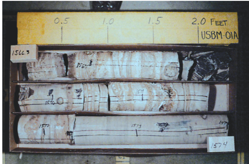
Figure 12. Drill core containing alternating beds of light-brown nahcolite and oil shale. White crystalline aggregate of nahcolite located in right part of upper piece of core. Recovered core from the U.S. Bureau of Mines 01A (C0334) borehole (1,566.5 ft to 1,574 ft). Core is located at the U.S. Geological Survey's Core Research Center, Denver, Colo.
