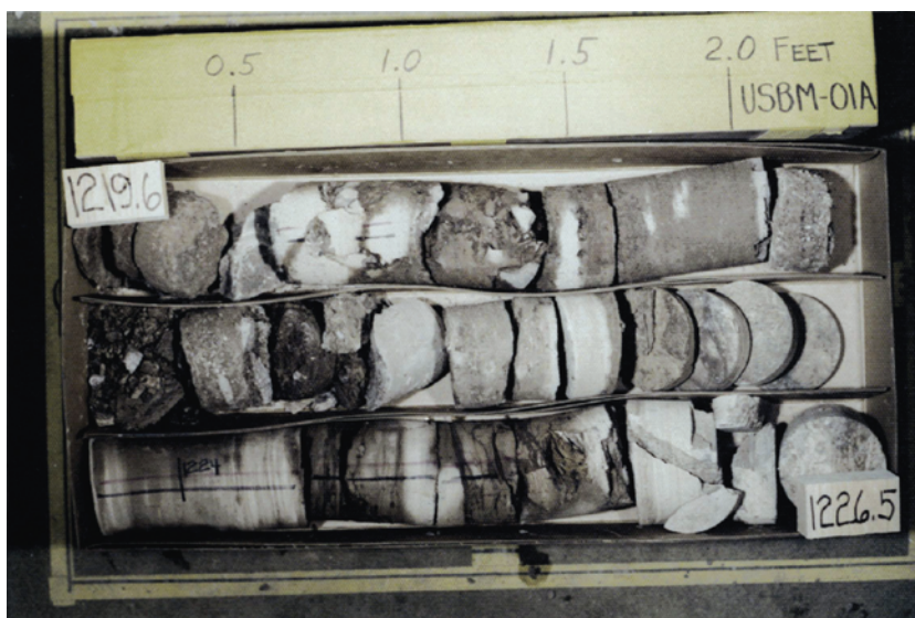
Figure 14. Drill core containing collapsed breccia and brown nahcolite and oil shale. Recovered core from the U.S. Bureau of Mines 01A (C0334) borehole (1,219.6 ft to 1,226.5 ft). Core is located at the U.S. Geological Survey's Core Research Center, Denver, Colo.
