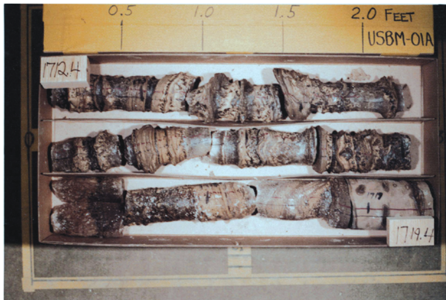
Figure 13. Drill core containing alternating beds of deeply dissolved halite and brown resistant wafer-like nahcolite. Recovered core from the U.S. Bureau of Mines 01A (C0334) borehole (1,512 ft to 1,519.4 ft). Core is located at the U.S. Geological Survey's Core Research Center, Denver, Colo.
