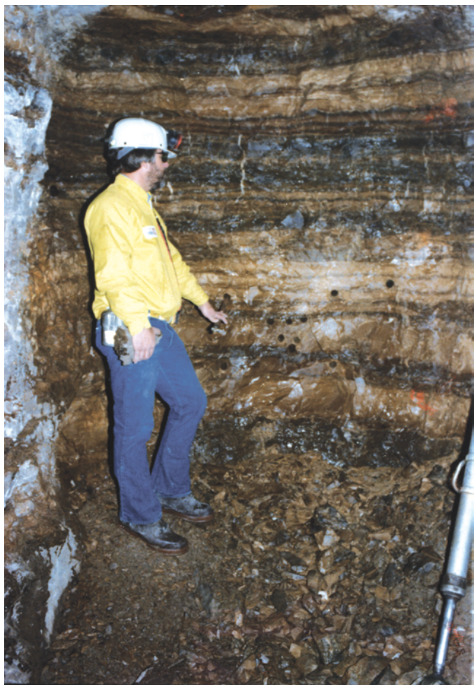
Figure 7. An excavated face in the Horse Draw Mine, third level, U.S. Bureau of Mine's deep-shaft project (1,834 ft to 1,844 ft). Channel sample analyses of face from roof to floor: nahcolite, 63 weight percent; dawsonite, 3.5 weight percent; oil yield, 12.3 gallons per ton; water, 16.3 gallons per ton; spent shale percent, 85.2; and percent gas plus loss, 3.3. Shaft drilled, with a 10-ft-diameter composite drill bit (see fig. 6). Photograph was taken in 1979 by Robert Bolhmar (U.S. Bureau of Mines).
