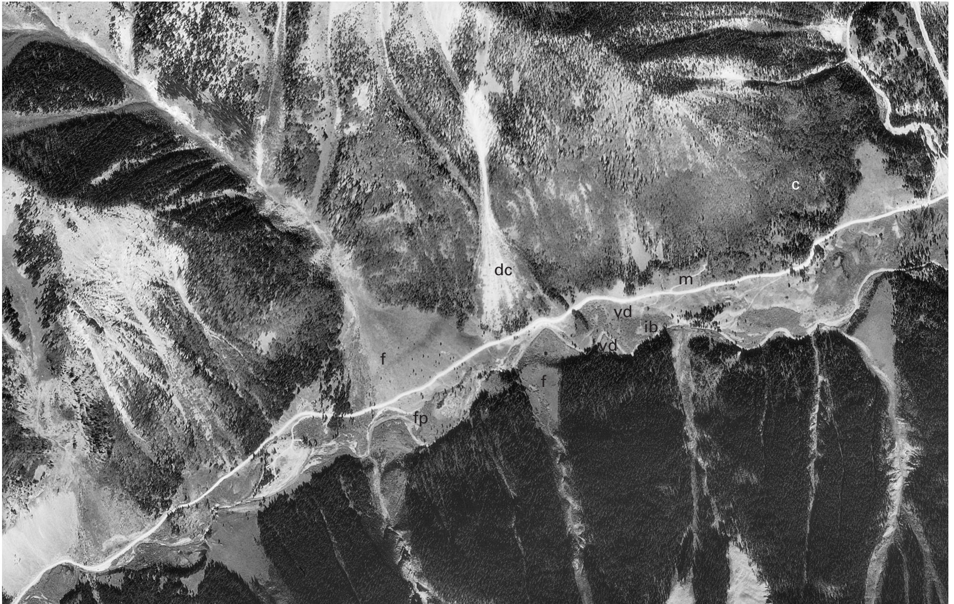
50. Fan (f), debris cone (dc), valley (vd), floodplain (fp), glacial till (m), iron bog (ib), and colluvial (c) deposits. Vertical digital orthophoto in the South Fork Mineral Creek drainage.
