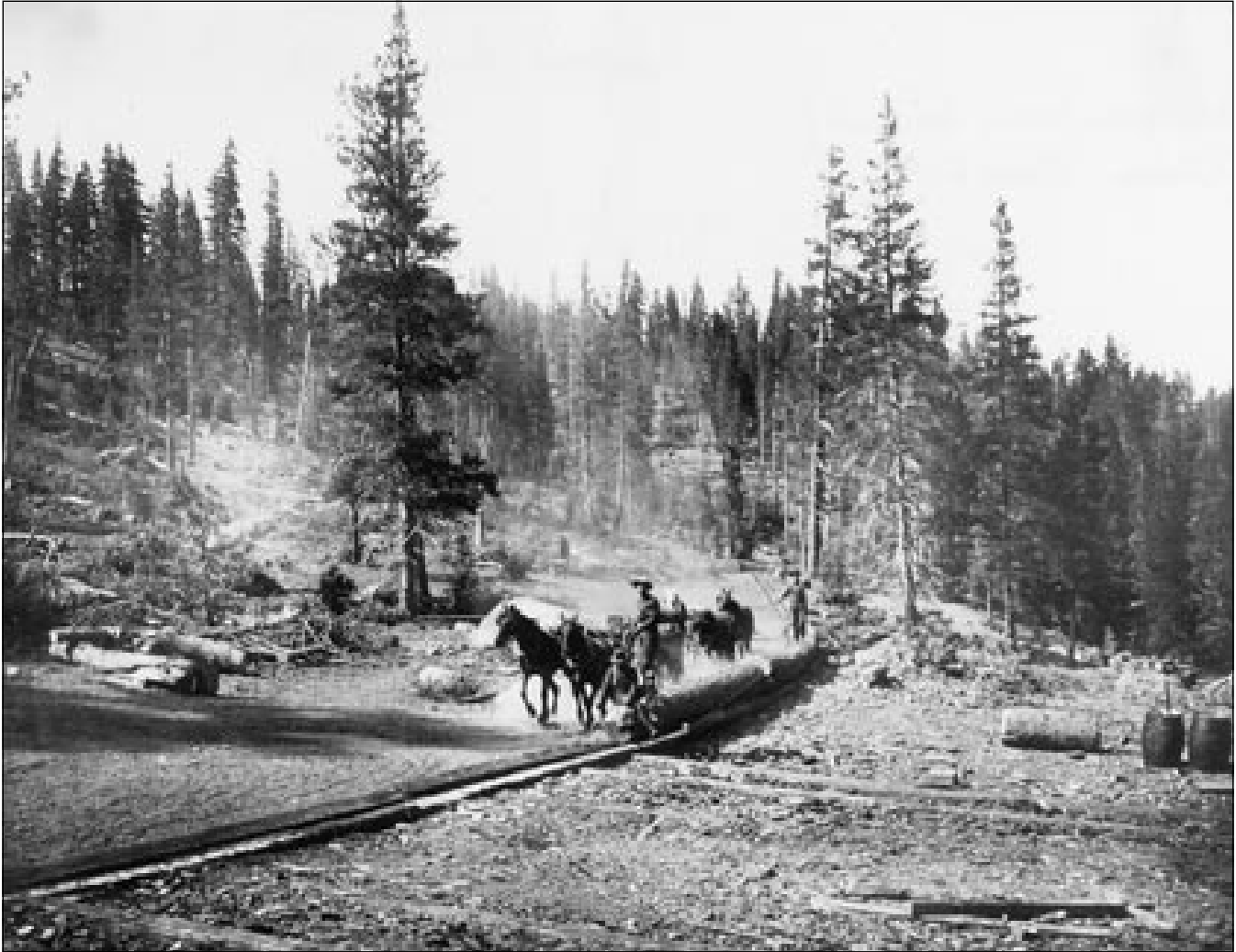
Turn-of-the-century logging in the Truckee River basin around Lake Tahoe used animals, narrow gauge railroads, and water flumes to haul out logs. Extensive areas in this region of mixed conifer forest had most of the tree cover removed. (Courtesy of Searles Historical Library/ J. Morse.)
