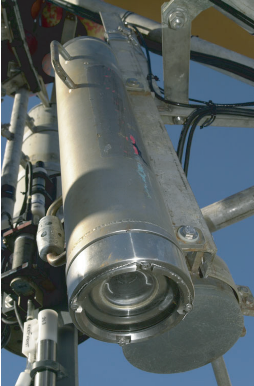
Figure 13G. Photograph of Benthos 35 mm underwater camera mounted on tripod frame (see figure 13A for photograph of tripod).
