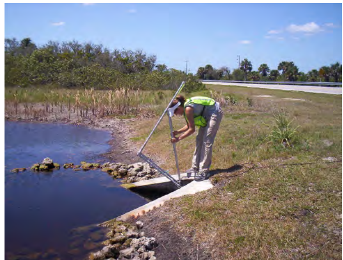
Figure 5. ADVM culvert installation (photograph by Lars Soderqvist, U.S. Geological Survey).
