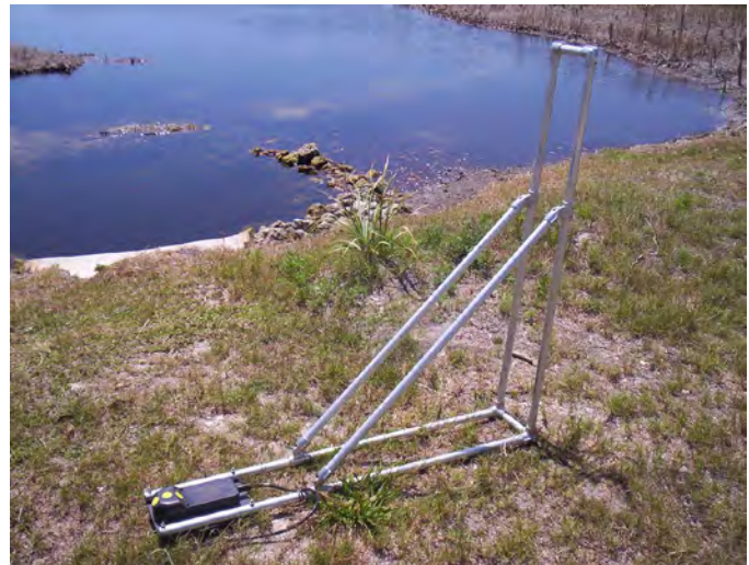
Figure 4. ADVM removable mount for culvert discharge measurements (photograph by Lars Soderqvist, U.S. Geological Survey).
