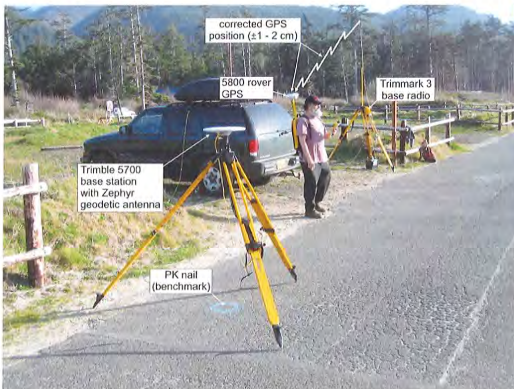
Figure 5. The Trimble 5700 base station antenna located over a known reference point at Cape Lookout State Park. Corrected GPS position and elevation information is then transmitted by a Trimmark III base radio to the 5800 GPS rover unit.
