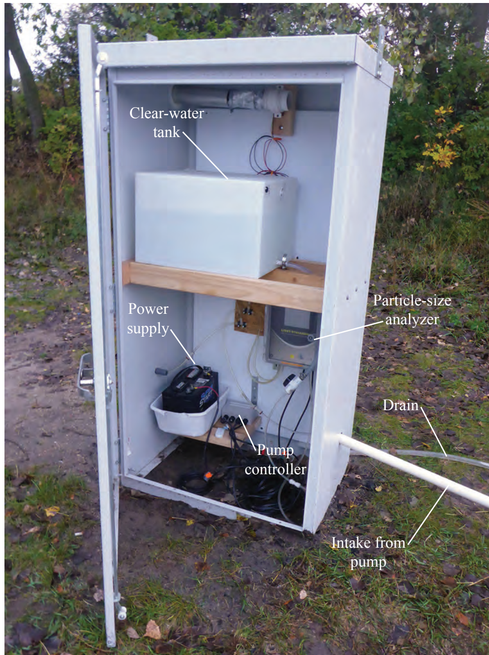
Figure 3. Sediment particle-size analyzer housing and instrumentation downstream from Spencer Dam, Nebraska.
