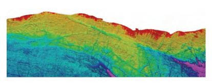
Beautiful rocky coastline off the west coast of Scotland. Data collected using an F185R+™ and an R2Sonic 2024. This data was acquired in very challenging conditions - a sea state 4 with typical swell of 4.0m with up to +-16 degrees of pitch and roll. The extremely accurate performance of the F185R+™ meant no editing of MBES data required. Image courtesy of Aspect Land & Hydrographic Surveys.
