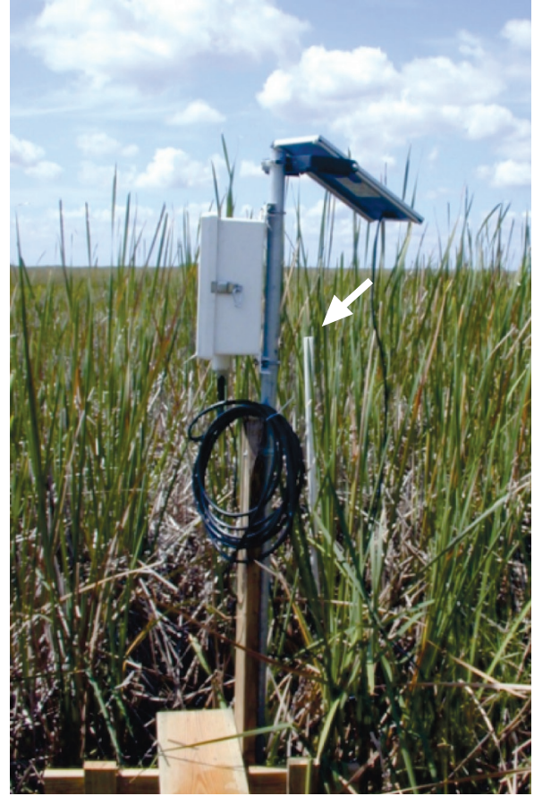
Figure 2. Thermistor string (attached to PVC pipe in center background indicated by arrow) deployed in a dense cattail area at NP202 in Shark River Slough, Everglades National Park, Florida.
