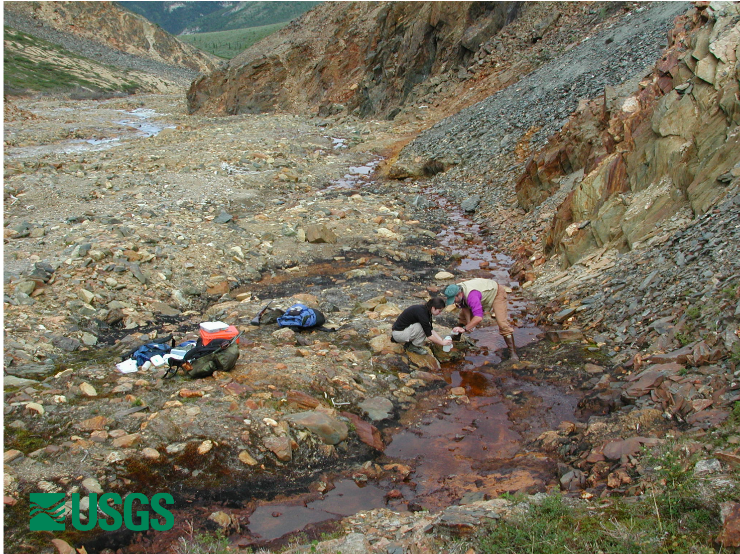
Photo 03BF008-1. View to NE of sample site; acid spring on the E side of Red Mountain Creek; pH 3.0, conductivity 3410 \mu\text{S}/\text{cm} .
