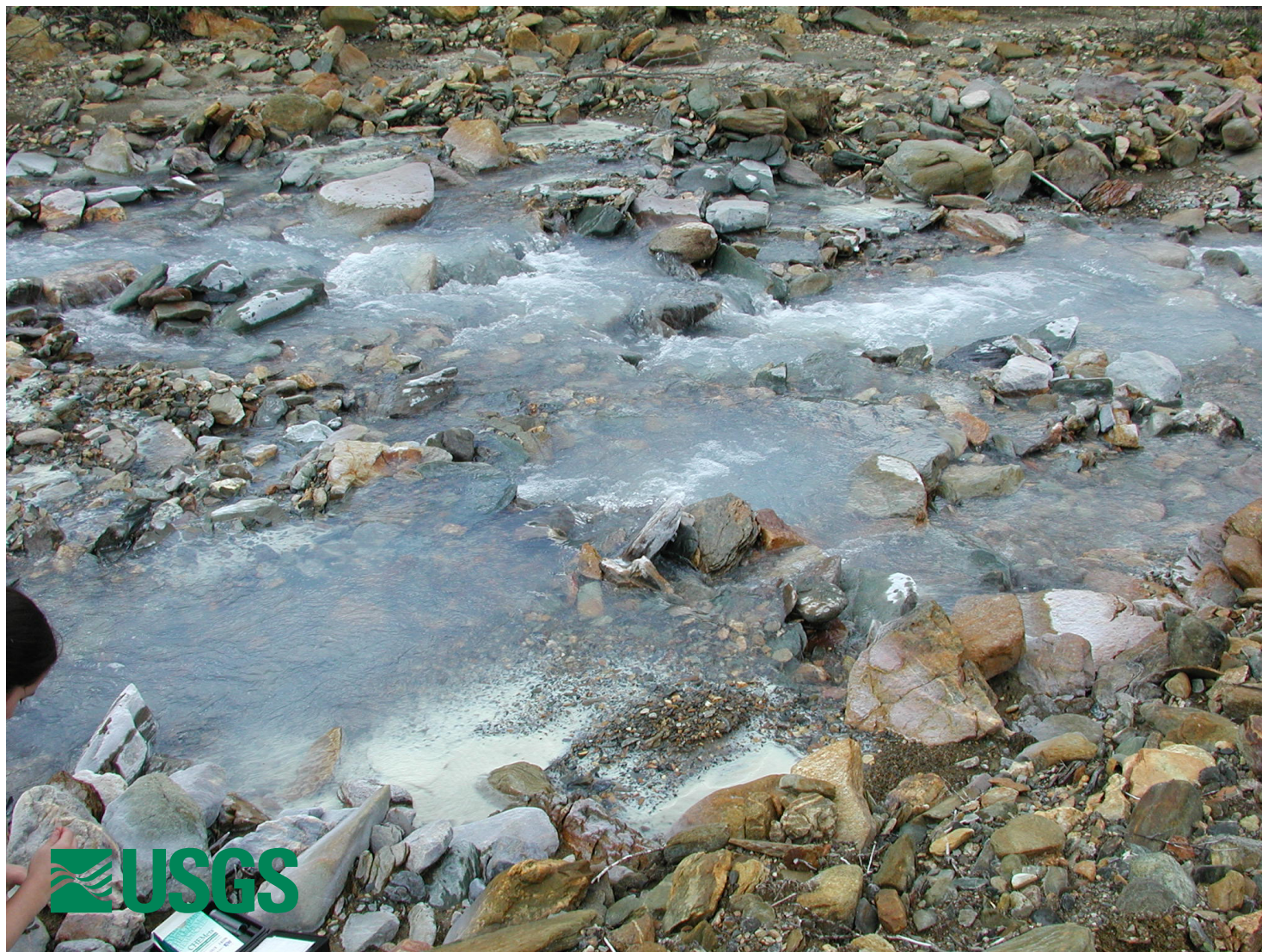
Photo 03BF009-1. Sample site, Red Mountain Creek with abundant Al floc; just downstream of exposed altered rocks; pH 4.6, conductivity 1200 \mu\text{S}/\text{cm} .
