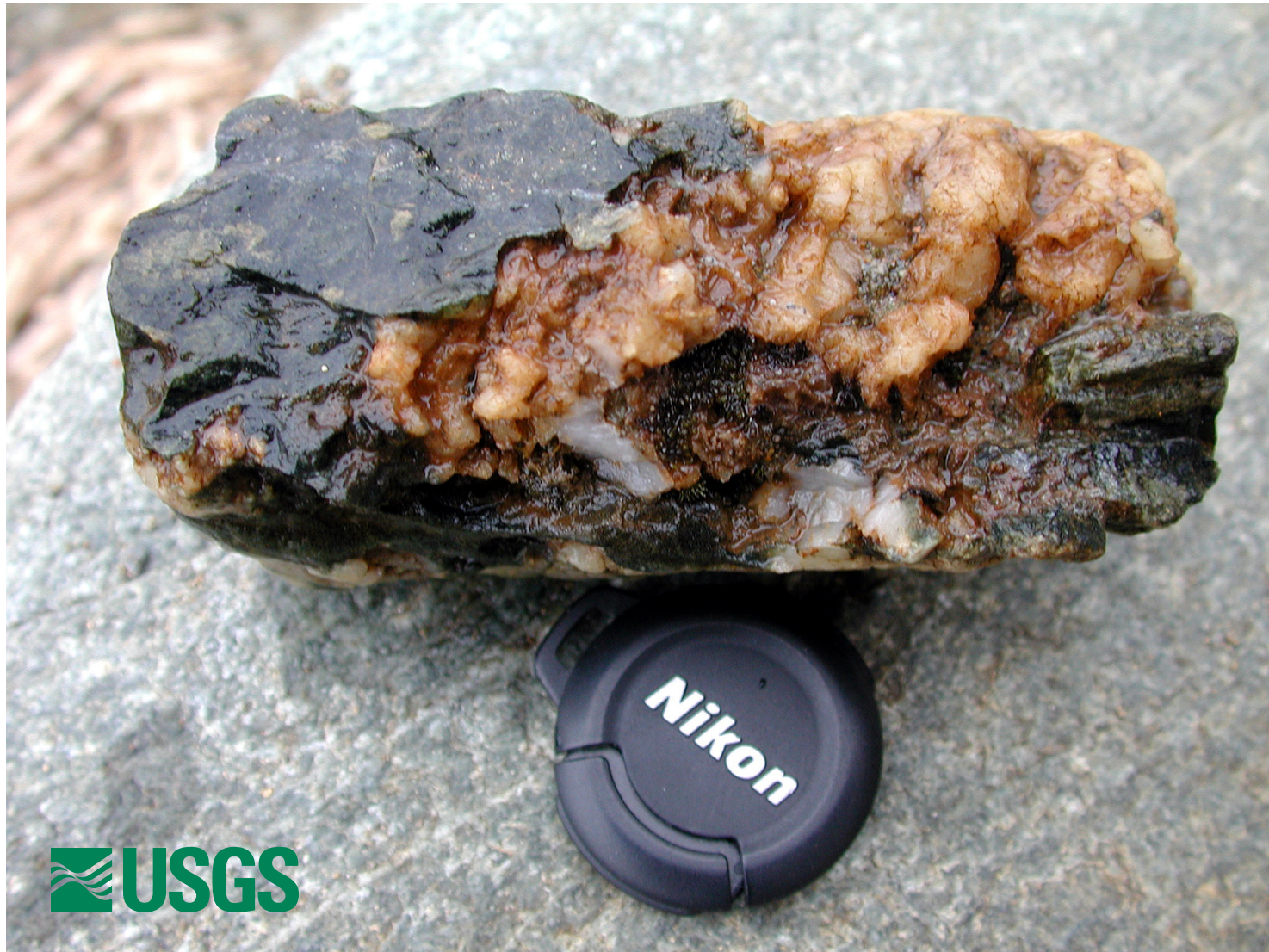
Photo 03BF011-2. Alluvial quartz-calcite vein cobble with calcite completely gone (consumed by acidic stream water) leaving irregular vugs.
