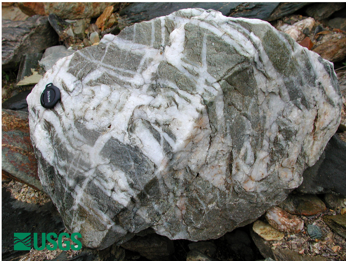
Photo 03BF014-3. Well-developed stockwork in colluvial boulder from just upstream of sample site.
