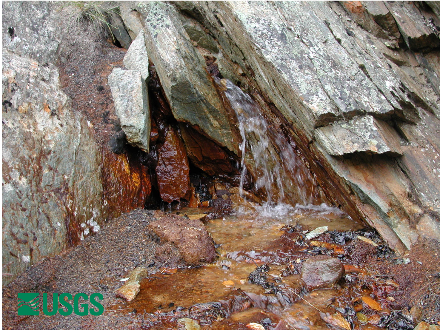
Photo 03BF015-1. Sample site, acid spring in fracture zone at mouth of Lago Creek; pH 2.7, conductivity 2920 \mu\text{S}/\text{cm} .
