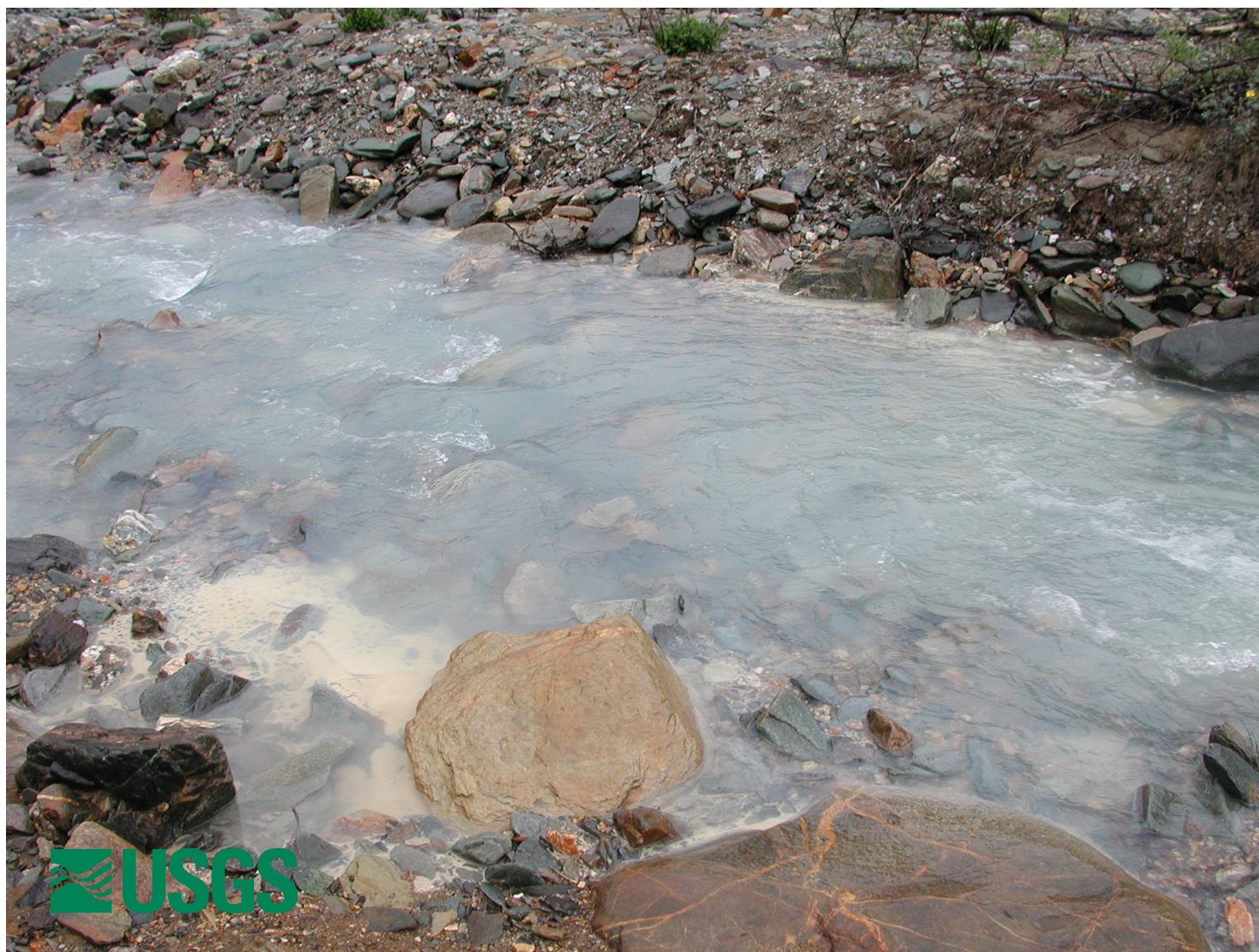
Photo 03BF017-1. Sample site, Red Mountain Creek at mouth, with abundant Al floc settled in calm areas; pH 4.2, conductivity 1180 \mu\text{S}/\text{cm} .
