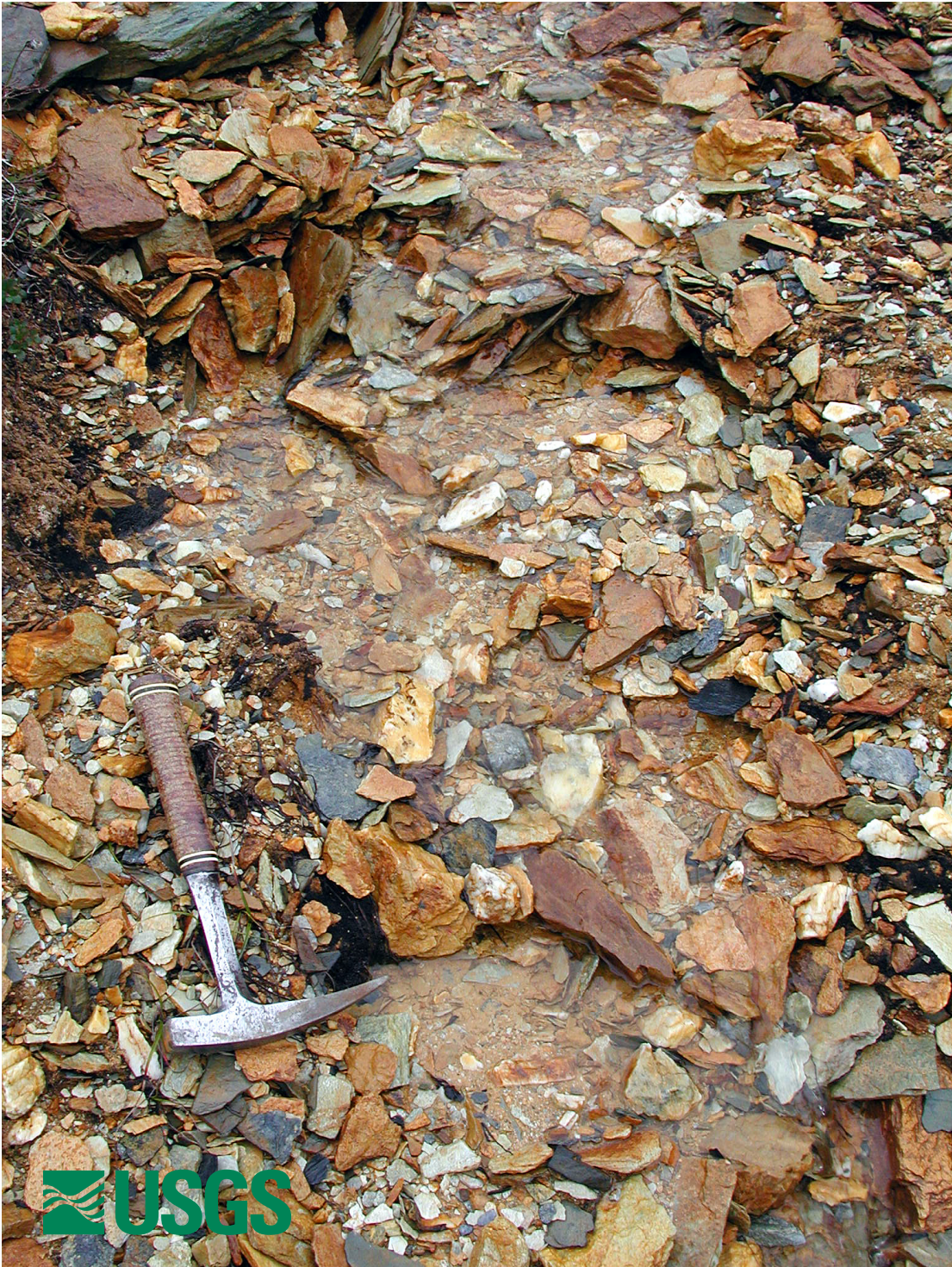
Photo 03BF022-1. Sample site, acid spring on W side of Red Mountain saddle; pH 2.5, conductivity 2520 \mu\text{S}/\text{cm} .
