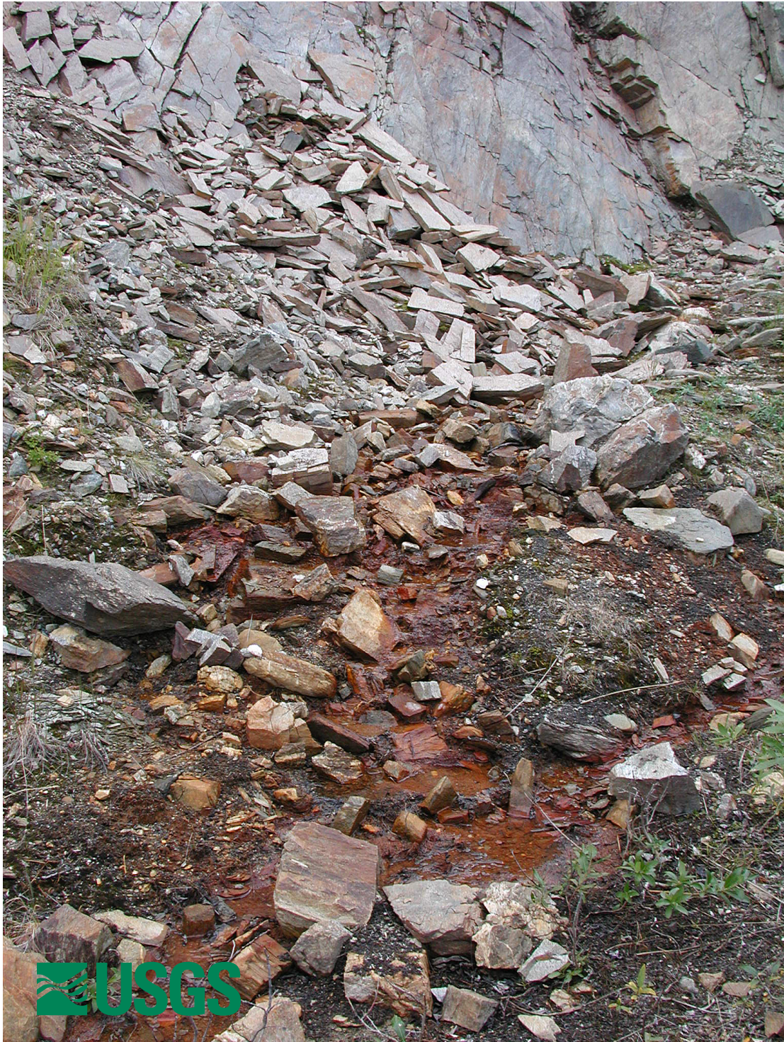
Photo 03BF029-1. Sample site, spring on E side of Foster Creek below Discovery Zone; pH 5.1, conductivity 878 \mu\text{S}/\text{cm} .
