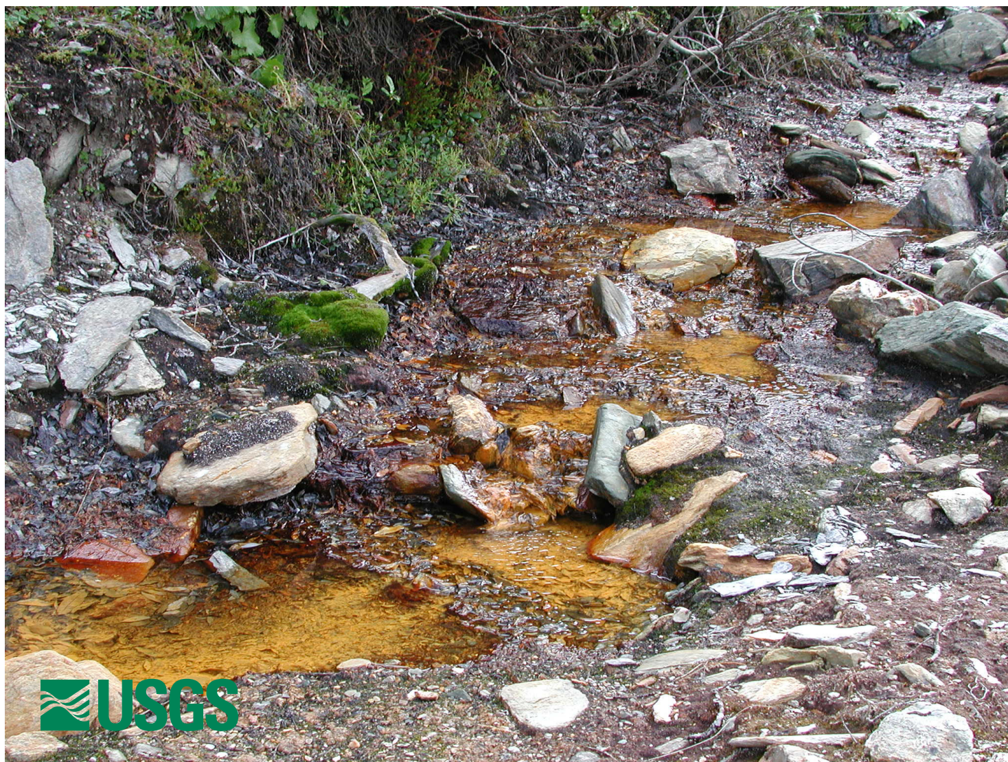
Photo 03BF030-1. Sample site, acid spring on E side of Foster Creek downstream of Lago Creek; pH 3.4, conductivity 2930 \mu\text{S}/\text{cm} .
