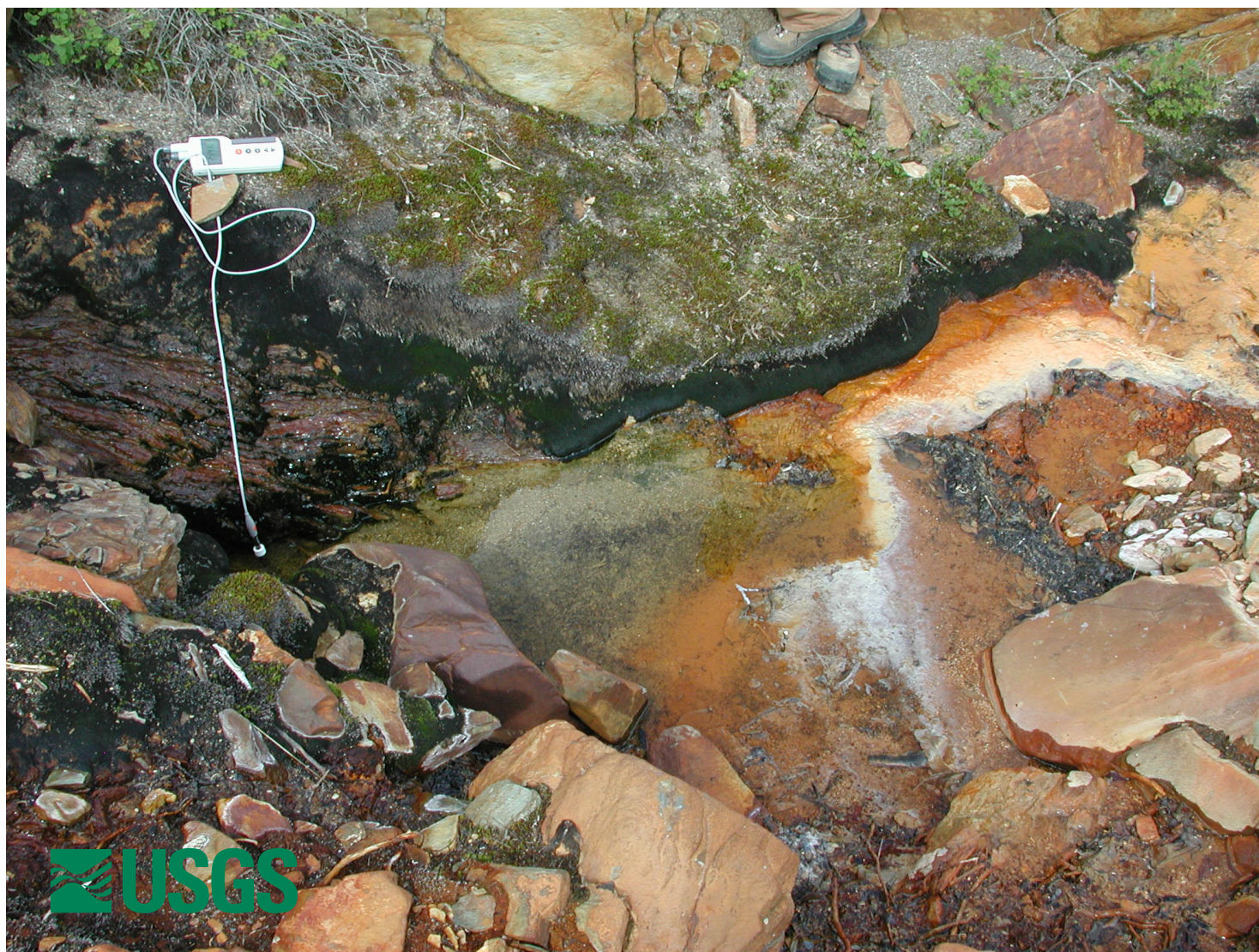
Photo 04BF051-1. Sampled spring along Lago Creek, Red Mountain area; pH 2.4, conductivity 2500 \mu\text{S}/\text{cm} . Re-occupation of sample site 03BF023.
