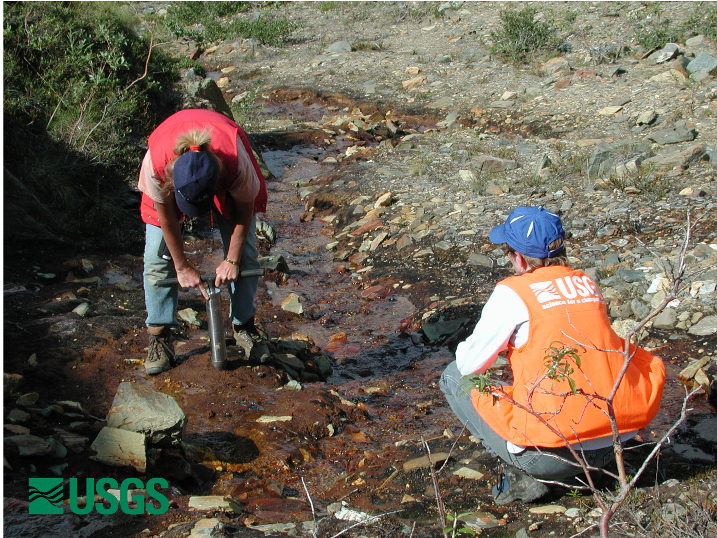
Photo 04BF054-2. NF and JEH coring ferricrete at spring sample site.
