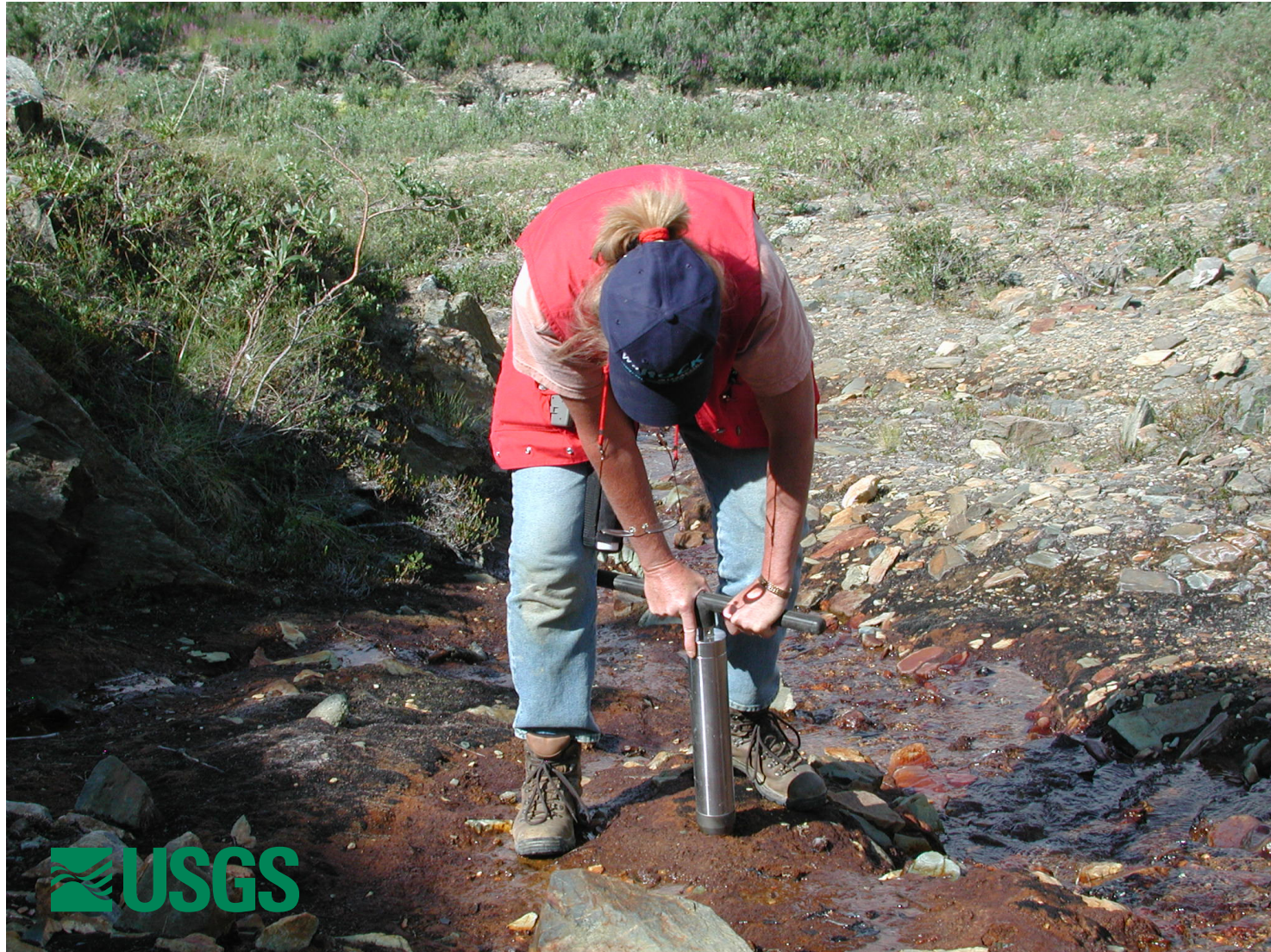
Photo 04BF054-4. JEH coring ferricrete at site.
