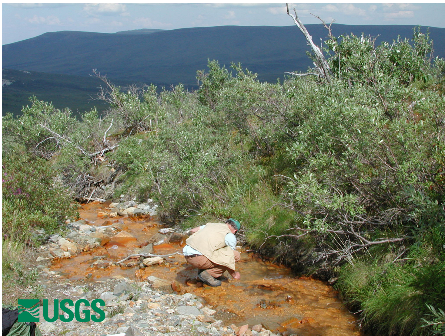
Photo 04BF060-1. Northerly view of PHB and sampled stream just downstream of lowermost outcrop of altered bedrock, lower Megan's Draw; pH 3.3, conductivity 1900 \mu\text{S}/\text{cm} .
