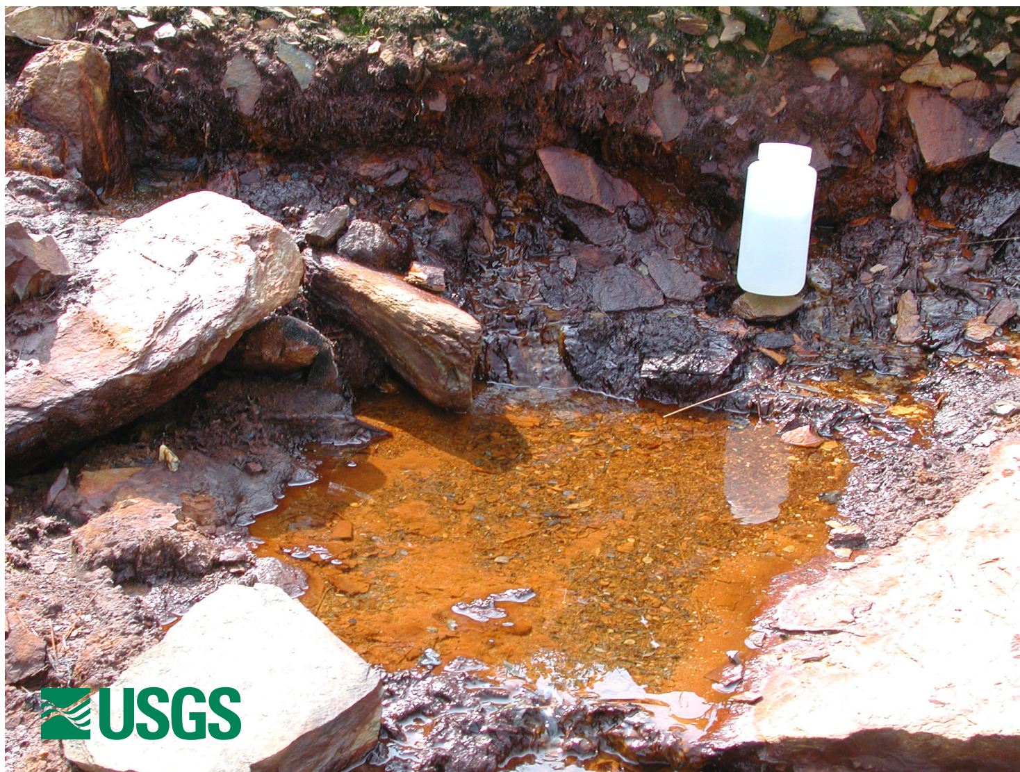
Photo 04BF063-1. Sampled spring along Red Mountain Creek; pH 3.2, conductivity 4800 \mu\text{S}/\text{cm} . Re-occupation of sample site 03BF008.
