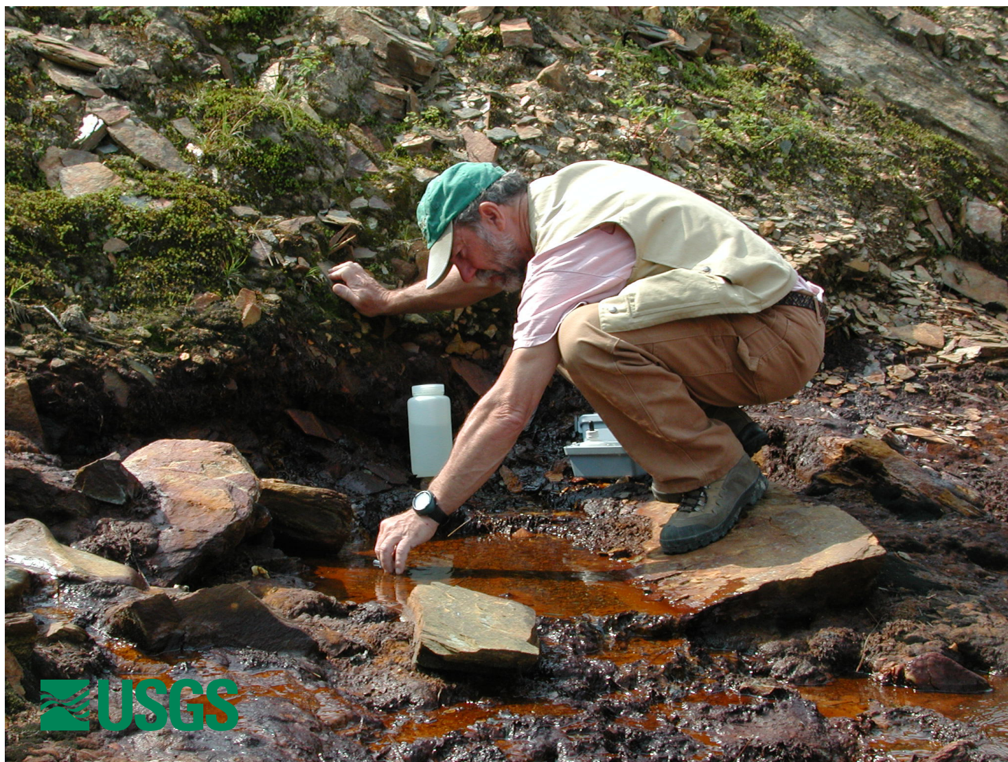
Photo 04BF063-2. PHB collecting water acidity data. Note heavy ferricrete precipitation.
