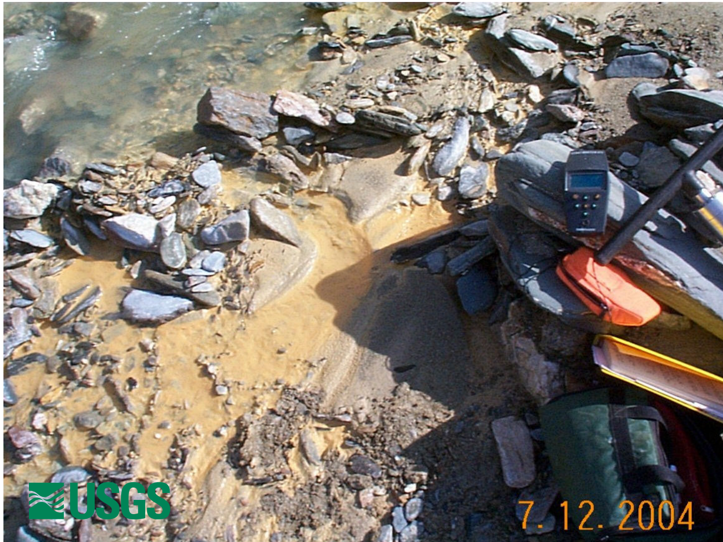
Photo 04JHBF14. Buff-colored Al- and Fe-rich precipitate along Foster Creek downstream of Lago Creek and all acidic inflows.
