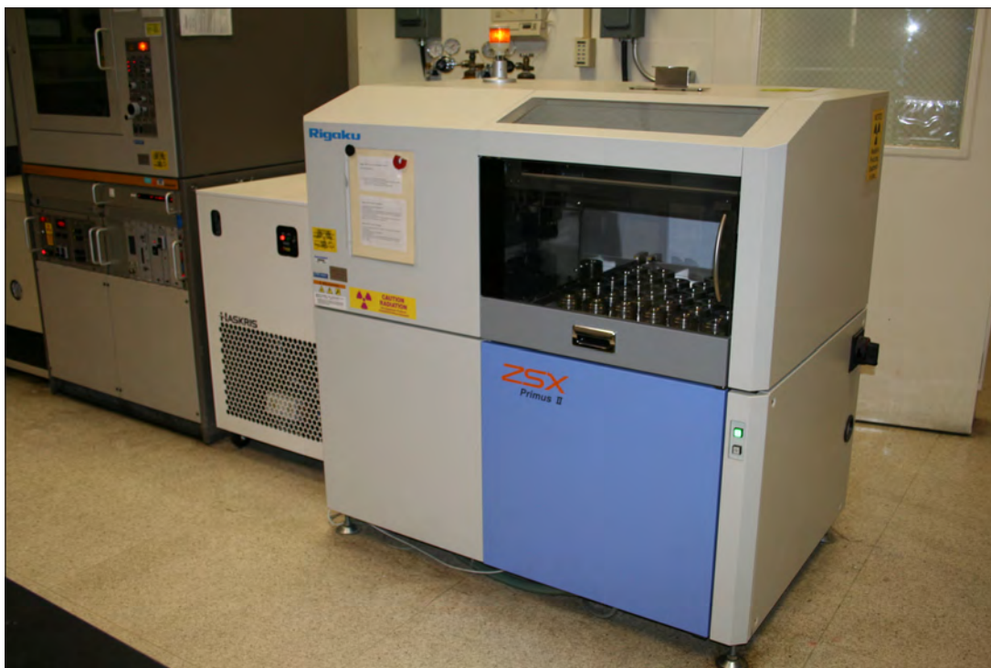
Figure 18. X-ray diffraction and fluorescence equipment. Machine shown on left is X-ray diffraction (XRD) analysis machine. Machine shown on right is X-ray fluorescence (XRF) analysis machine. Photograph taken by Emily C. Kluk, Los Alamos National Laboratory.
