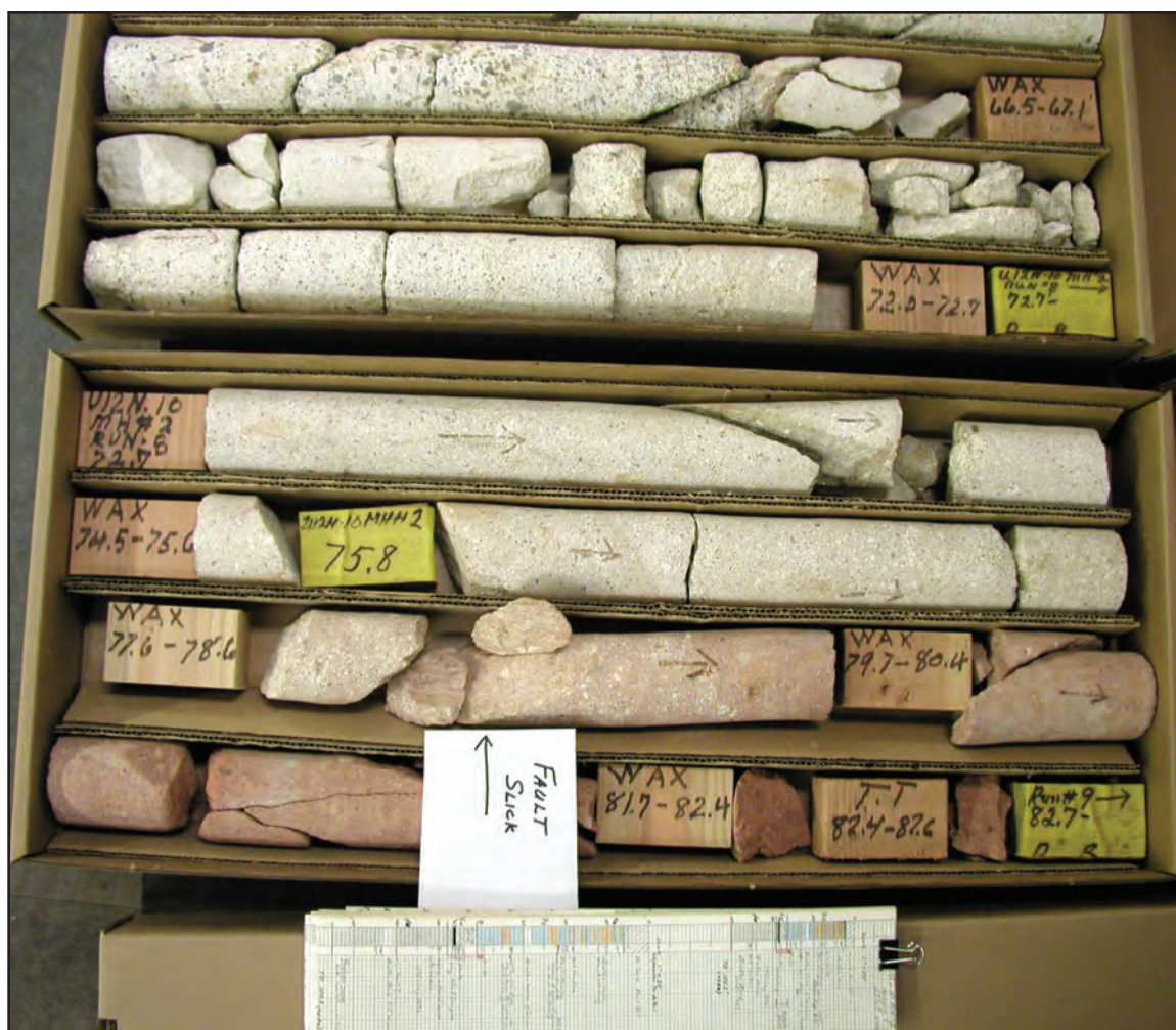
Figure 10. Example of subsurface fracture characteristics in vertical core hole MH-2 in floor of emplacement drift U-12n.10 at 303.77 feet from portal opening, Nevada National Security Site, Nye County, Nevada. Core sample shows slickensides and black staining on fracture surfaces at 79 feet. Photograph taken by Jerry Magner, U.S. Geological Survey.
