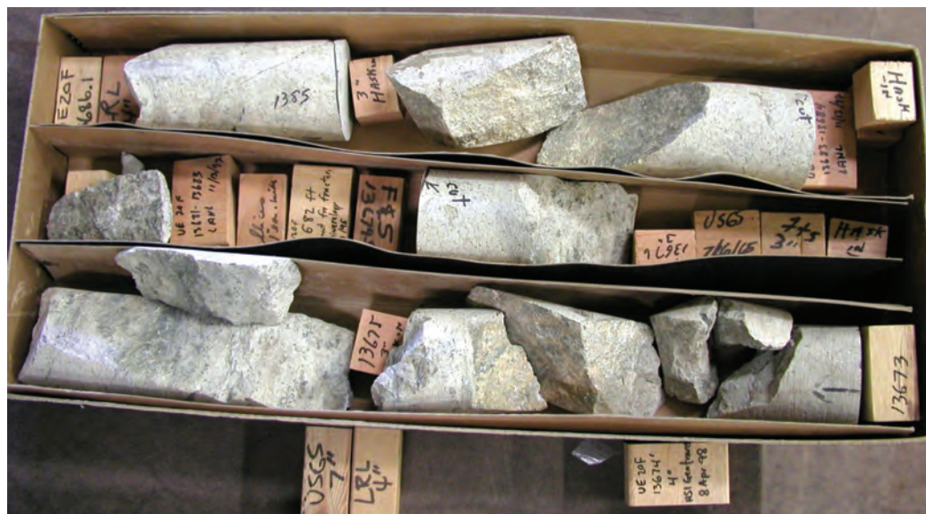
A. Subsurface core collected from bottom interval of exploratory hole UE-20f; deepest hole drilled at Nevada National Security Site. Core sample shows welded volcanic tuff from 13,670- to 13,686-foot interval. Wooden blocks indicate sections of core removed from U.S. Geological Survey Core Library. Photograph taken by Jerry Magner, U.S. Geological Survey.
