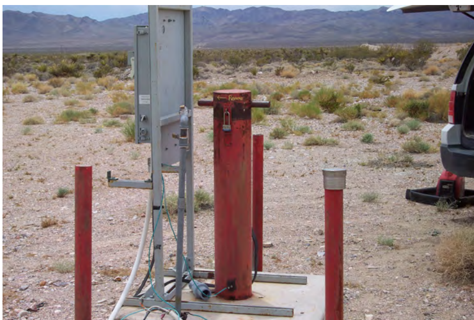
Figure 15. View facing west toward Specter Range of SM-23-1 monitoring hole located in Mercury Valley, Nye County, Nevada. Protective casing is 6-inch diameter and casing (not shown) is 4-inch diameter to a total depth of 1,332 feet. (Photograph taken by Terry R. Miller, U.S. Geological Survey.)
