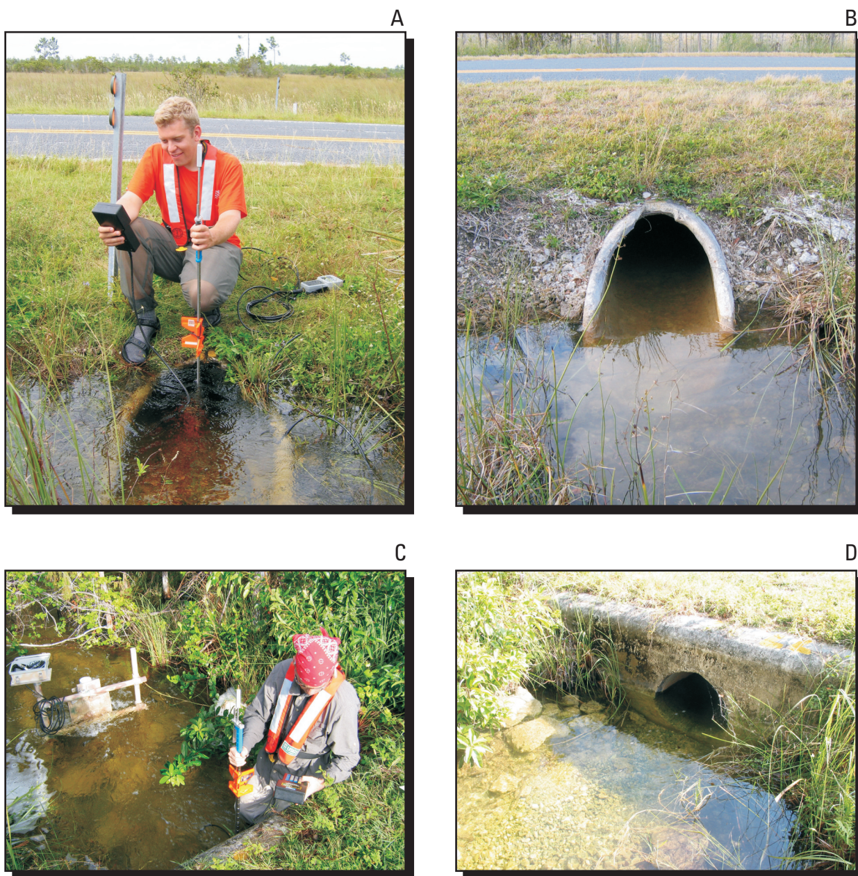
Figure 4. FlowTracker-ADV® meter mounted on wading rod to measure data at (A and B) culvert 34 and (C and D) culvert 77. The instrument interface was a handheld unit.
