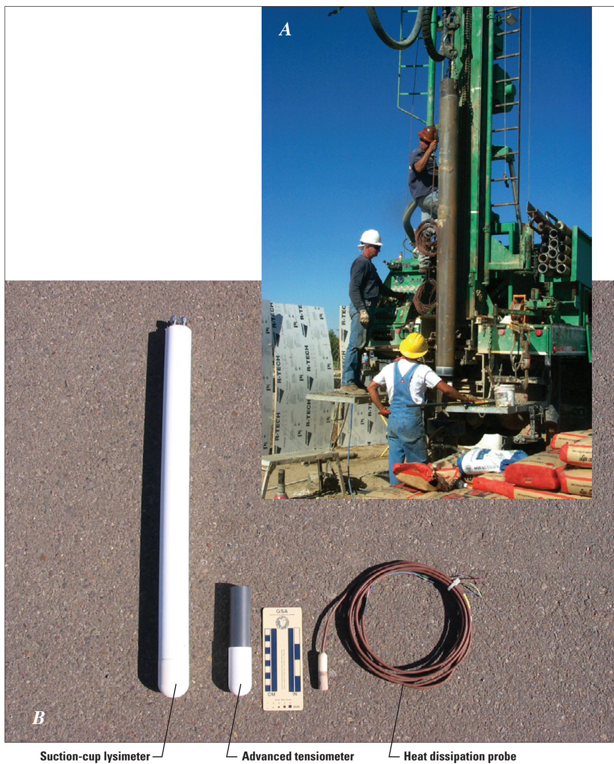
Figure 9. A, U.S. Geological Survey drill rig configured for ODEX drilling and B, selected instruments installed within the unsaturated-zone monitoring site at recharge ponds near Victorville, San Bernardino County, California.
