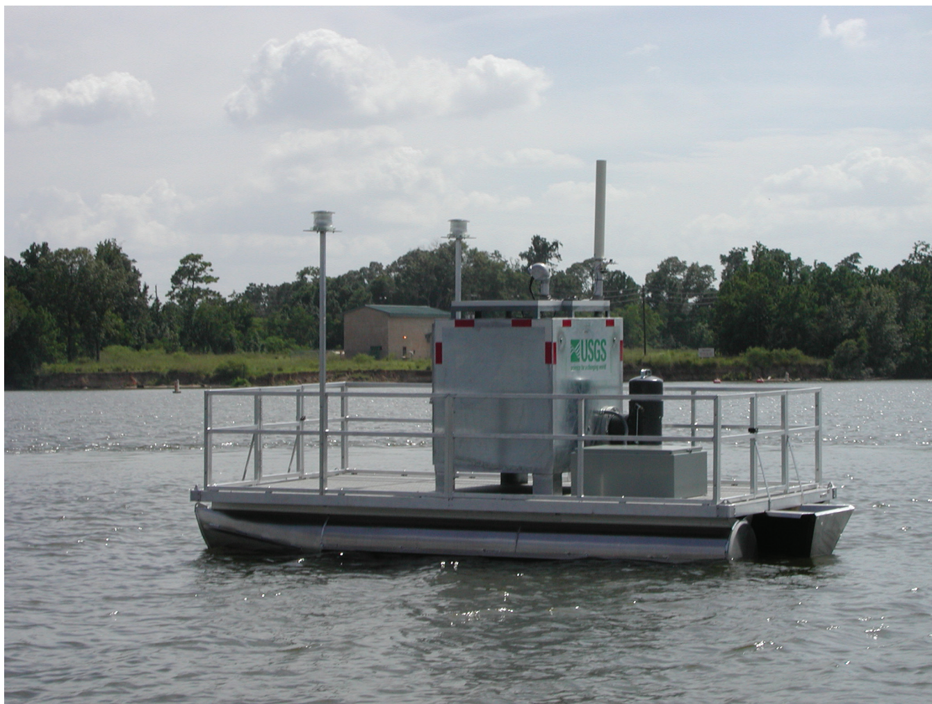
Figure 3. U.S. Geological Survey continuous water-quality monitoring system at site B on Lake Houston, station 295554095093401, Lake Houston at mouth of Jack's Ditch near Houston, Texas (photograph by T.D. Oden, August 14, 2006).
