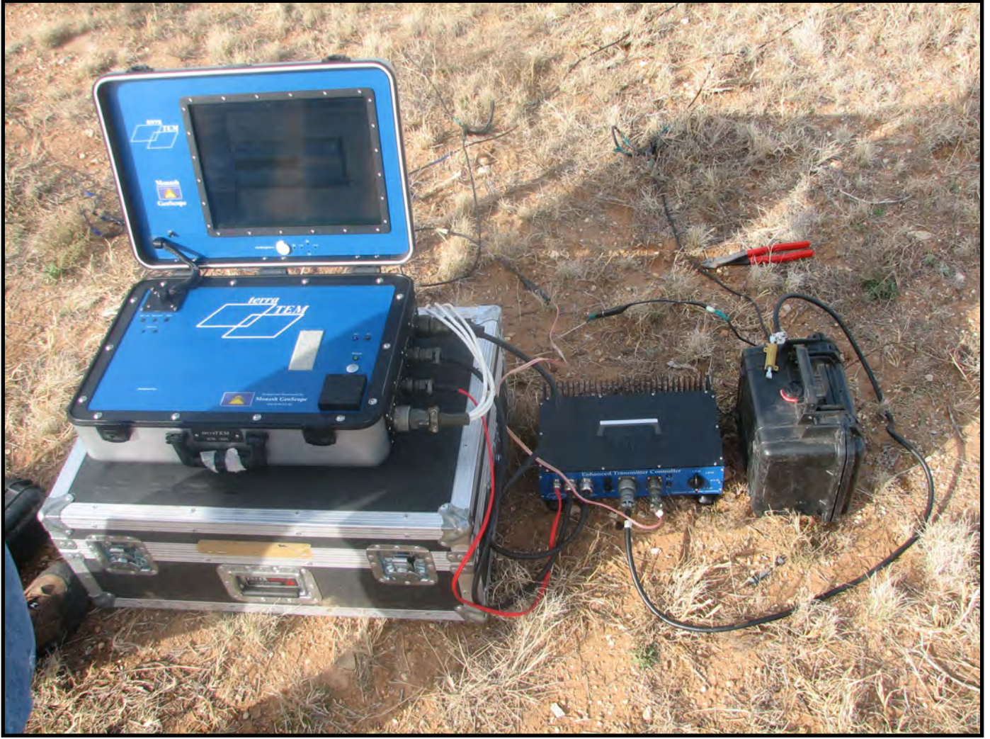
Figure 4. Alpha Geoscience TerraTEM time-domain electromagnetic system, which includes transmitter and receiver, current-limiting controller box, and battery pack.
