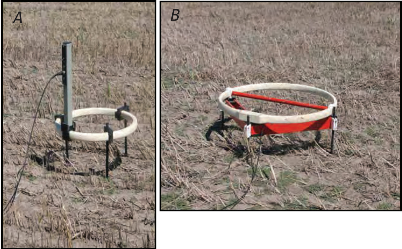
Figure 3. Photographs showing A , receiver coil (loop) for Geonics Protem-47, and B , receiver coil for Geonics Protem-57.
