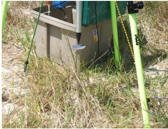
Figure 7. Photograph of the WHRN elevated benchmark cap.
