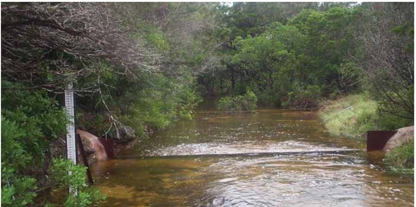
Figure 3. Streamflow channel and weir at site LC_{SW} (U.S. Geological Survey streamflow-gaging station 08180942 Laurel Canyon Creek near Helotes, Texas), Government Canyon State Natural Area, Bexar County, Tex., on June 29, 2004.
